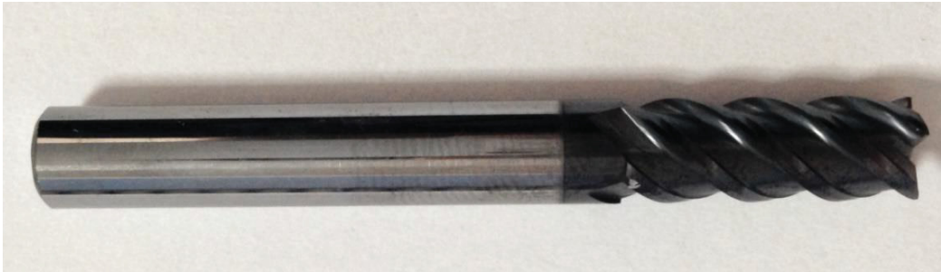
Figure 5.4 End-mill manufactured with CNC grinding machine.
