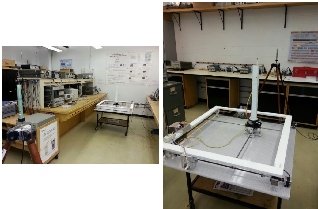
Figure 9.3: Experiment in the microwave lab H853. Measurement setup. The photo shows the xy positioner and the Styrofoam pole used to move the receive antenna.
