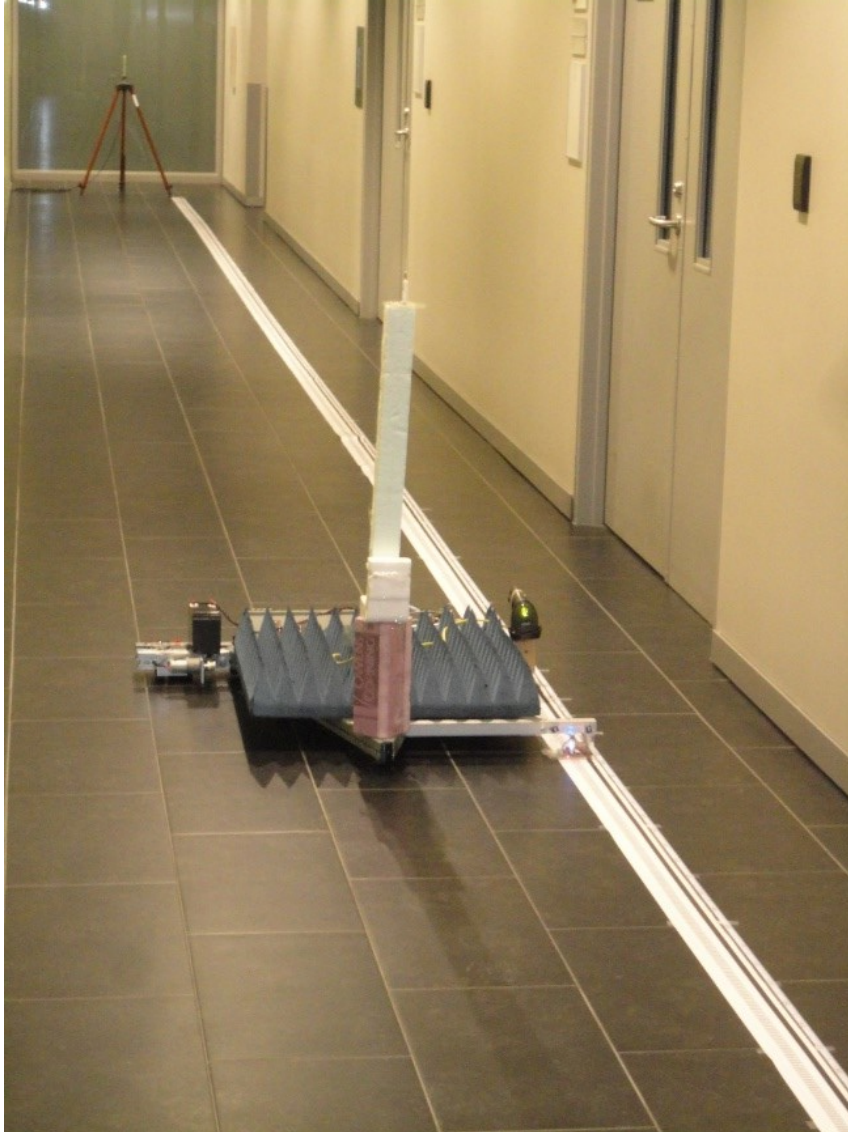
Figure 8.18: This figure shows the corridor on the 15th floor of the EV Building, and the line-follower “robot” carrying the receive antenna, with the transmit antenna in the background.
