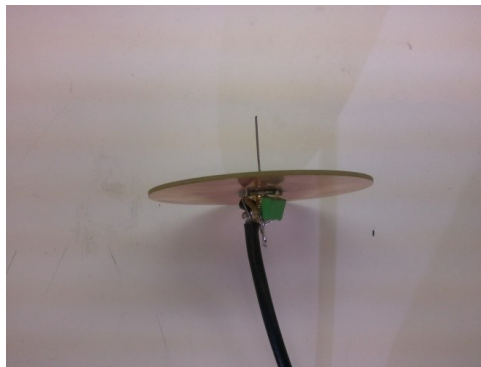
Figure 5.2: Monopole Antenna with a diode detector and an amplifier circuit.
