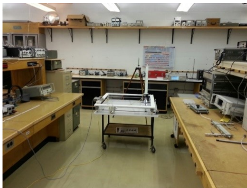
Figure 9.1: Microwave Lab on the 8th floor of the Hall Building. The photo shows that the file cabinet with instruments stored on top of them near the Tx. Both antennas are positioned at a height greater than the height of the file cabinet.
