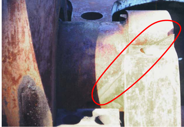
Figure 1.2: Sample failed engine crankshaft (in 45° due to torsional vibration) [12]
