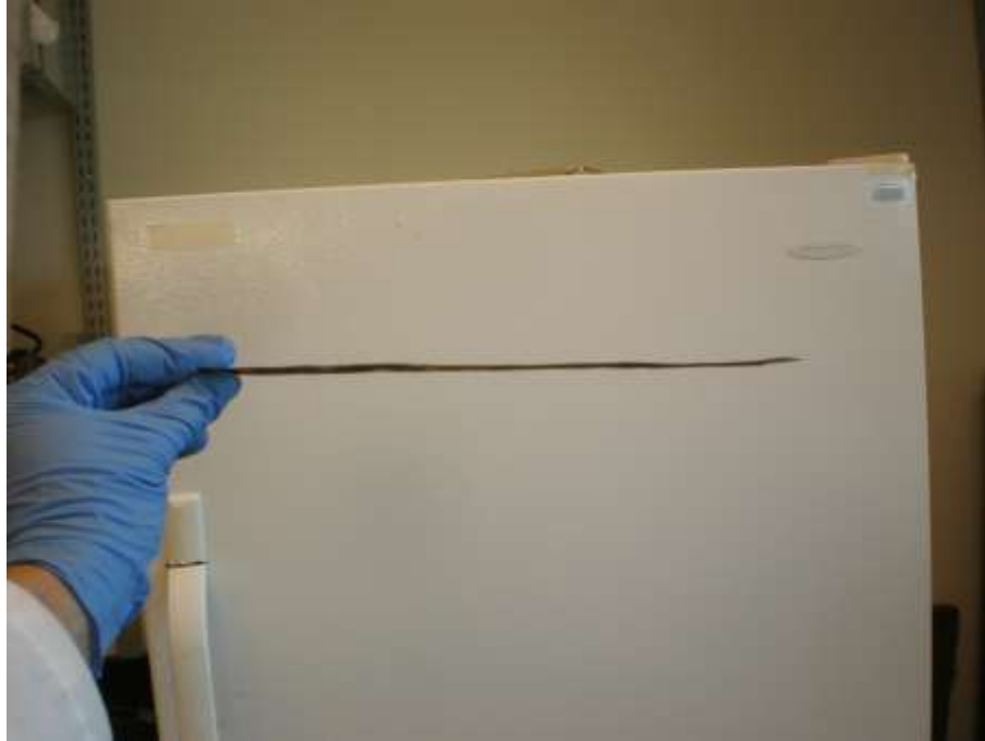
Fig. 3.6: New material - Carbon fibres with CNTs added with the aid of ultrasound: a) CNTs attached to carbon fibres; b) Increased stiffness of modified carbon fibres.
