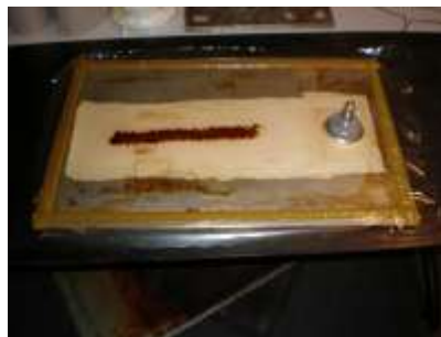
Fig. 3.10: Sample after curing in autoclave.
