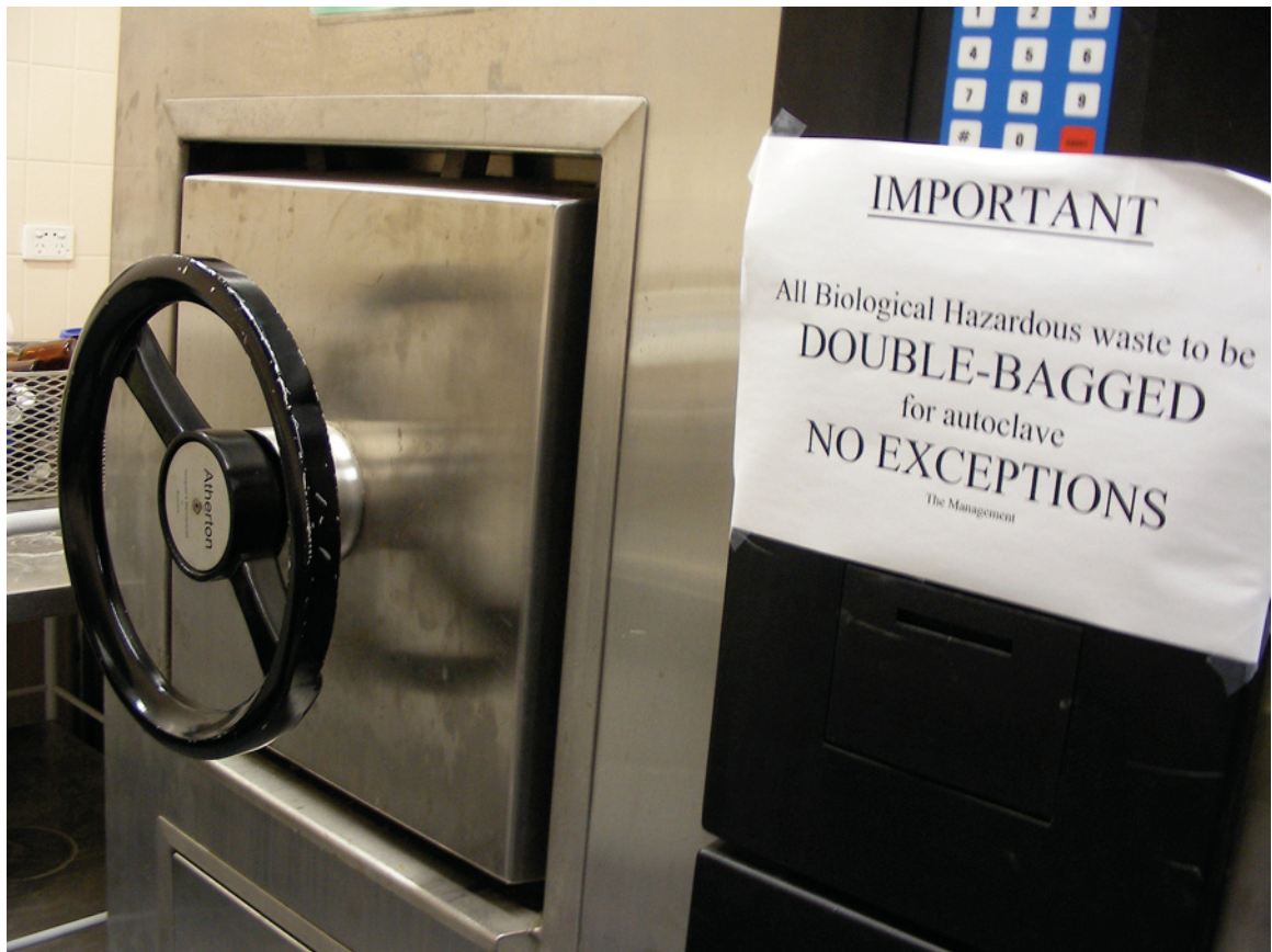
Fig. 21: Autoclave used to decontaminate and sterilize instruments Photograph credit: Tagny Duff (2008)
