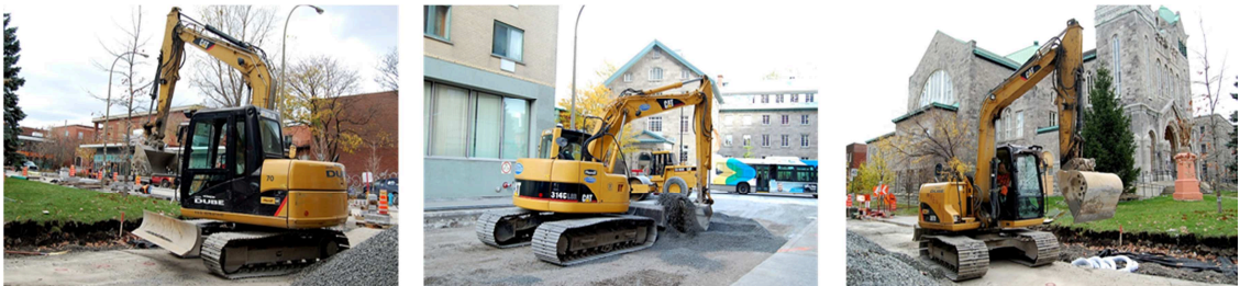
Small excavator: (a) CAT 307D, (b) CAT 314C, (c) CAT 307D (from left)
