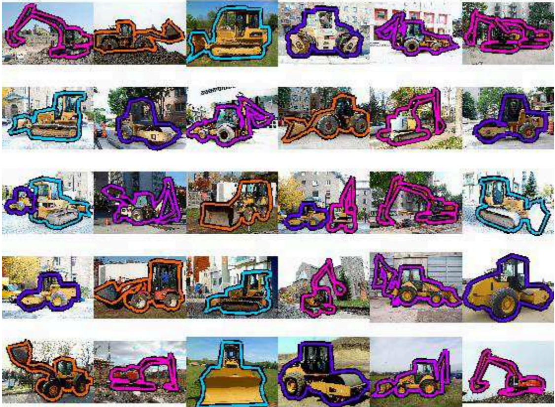
Figure 5-5: Training and test database created by the simple object detector with boosting method with the images of construction equipment
