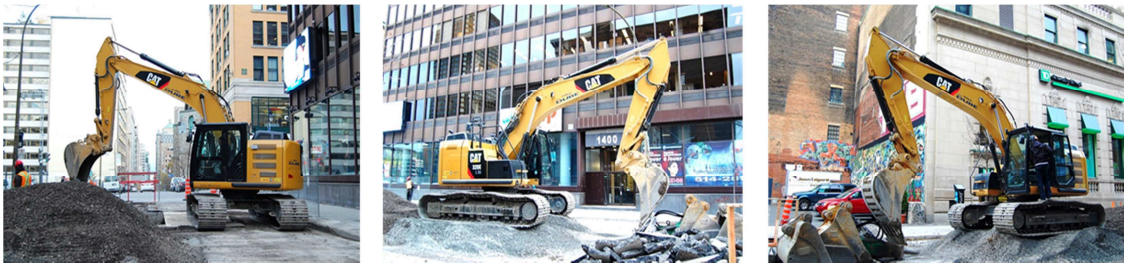
Medium excavator: (a) CAT 324D, (b) CAT 320E, (c) CAT 324D (from left)
