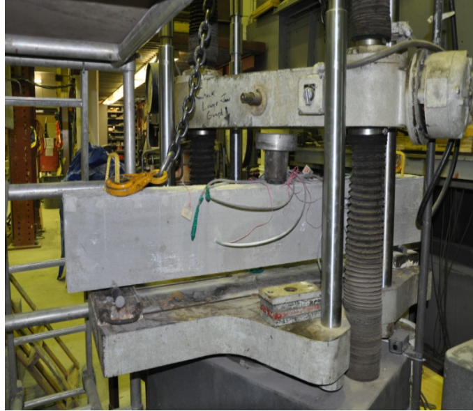
Figure 3-7 Preloading the beam
