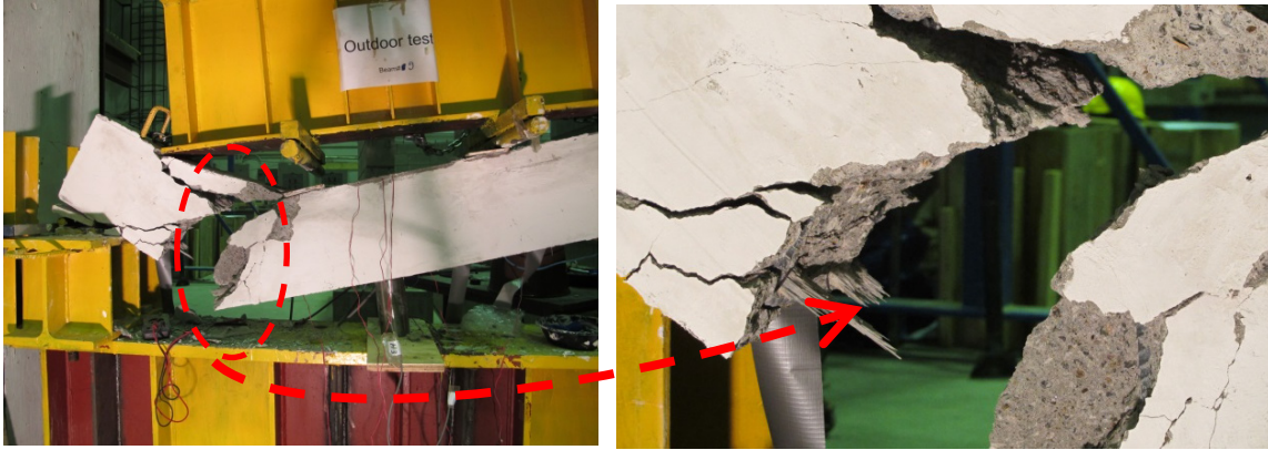
Figure 4-10 Typical shear-fracture in post failure loading of GFRP RC- beam in Outdoor
