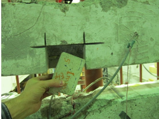
Figure 3-18 Cubic piece extracted by circular saw (embedded bar)
