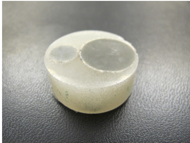
Figure 3-18 Cubic piece extracted by circular saw (embedded bar)
