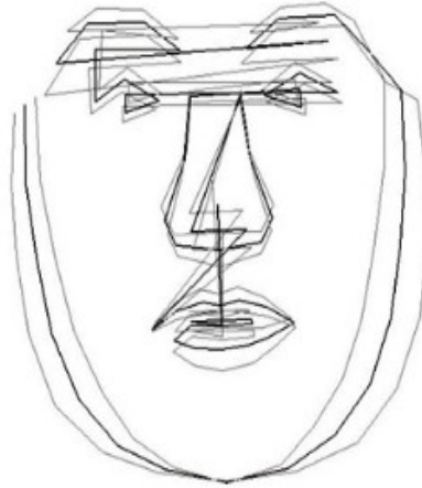
Figure 13: The mean face shape model (black line) and the variations on the model (gray lines)
