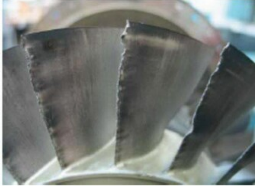
Figure 2.16: The effect of erosion on turbine blades [136].
