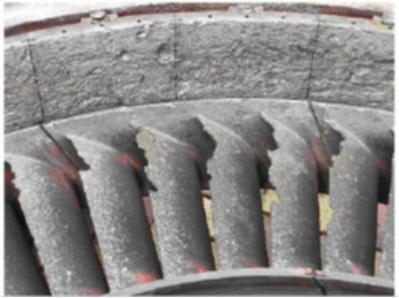
Figure 2.8: The effect of foreign object damage on gas turbine blades [119].
