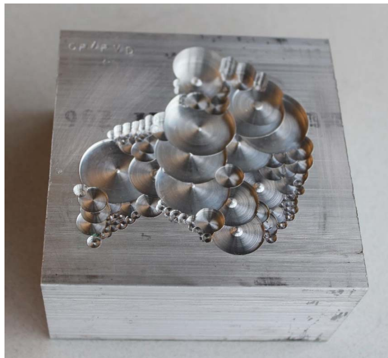
(b) Plunge milling roughing by CP algorithm with considering the depth of cut.
