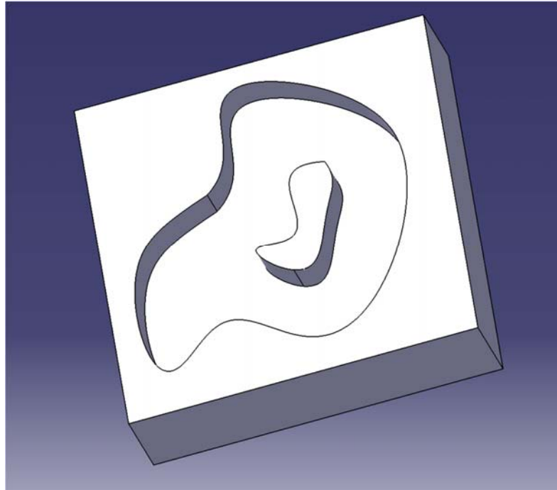
(a) CATIA model for pocket with island have free form boundary.
