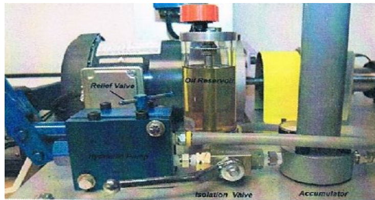
Figure 18 BPS hydraulic loading system
