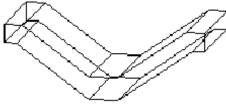
Isometric View – Sinusoidal iShell Footing Model.
