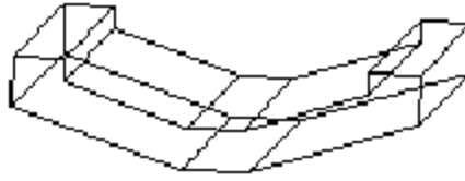
Isometric View – iShell Footing Model iS#1.
