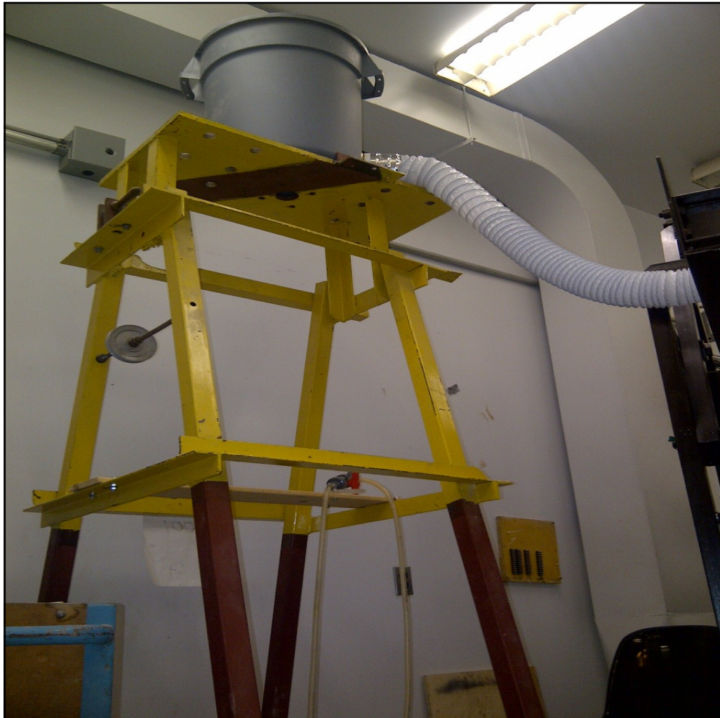
Figure 4.50. Elevated Storage Bin & Funnel System for Sand Pluviation.
