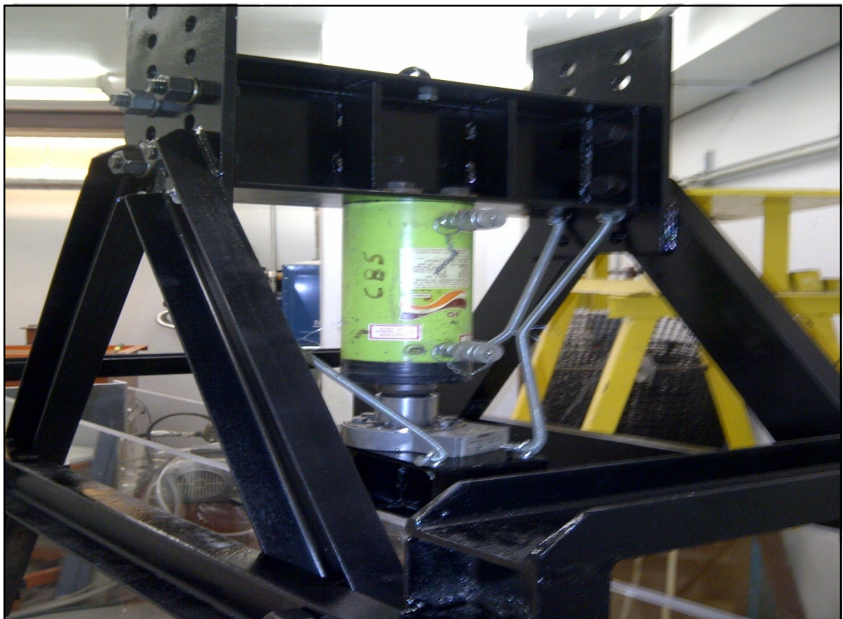
Figure 4.28. Loading Yoke, Load-Cell, Jack Cylinder and Ball-Pinion Setup.
