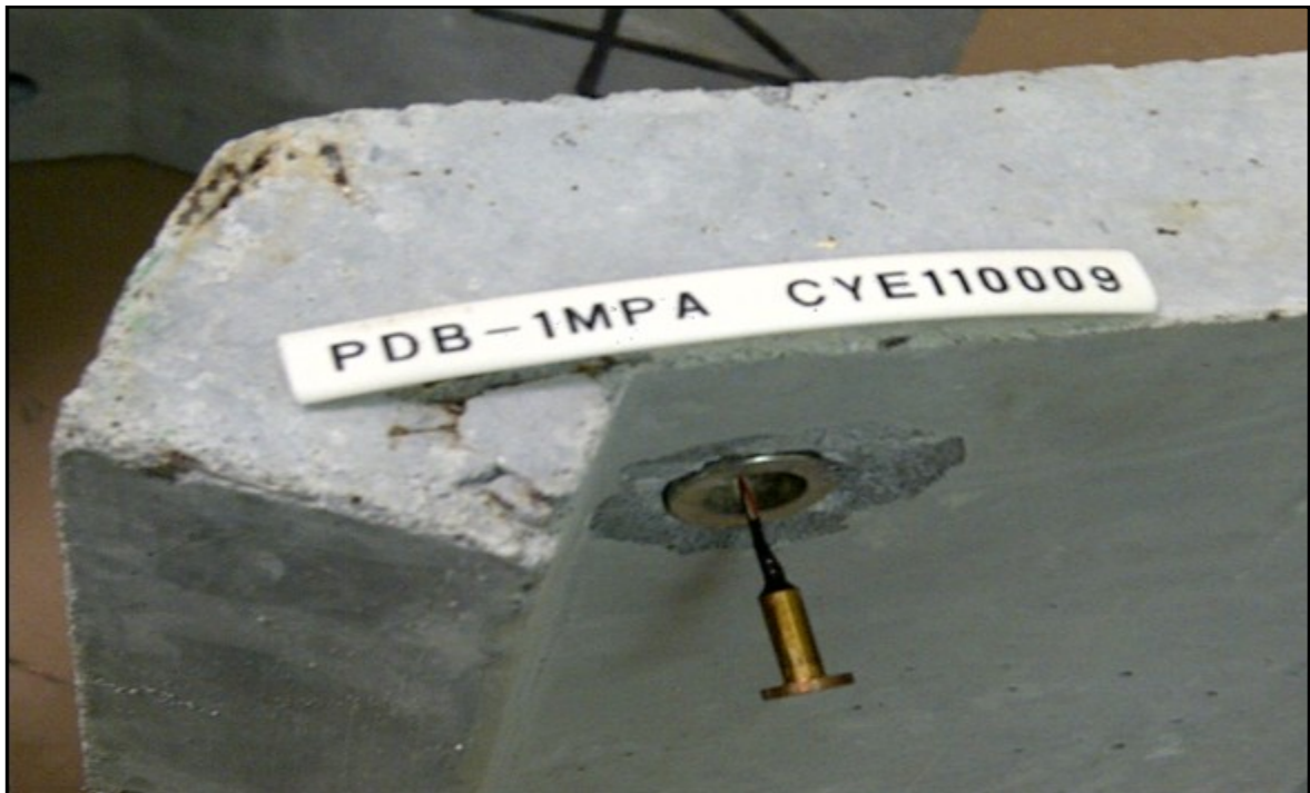
Figure 4.35. Pressure Transducer Insertion – iShell Footing Model.
