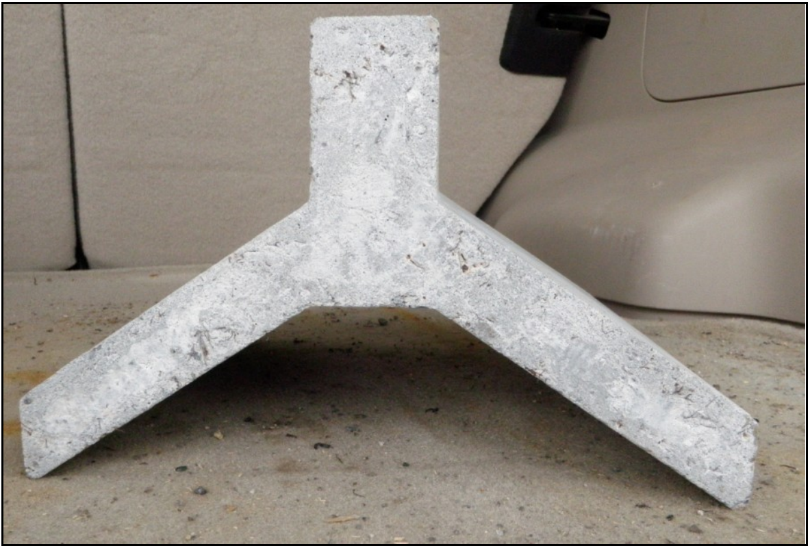
Figure 4.8. Upright Triangular Shell Model of iShell Mix Concrete, t_s = 25 mm, \theta = 34^\circ .
