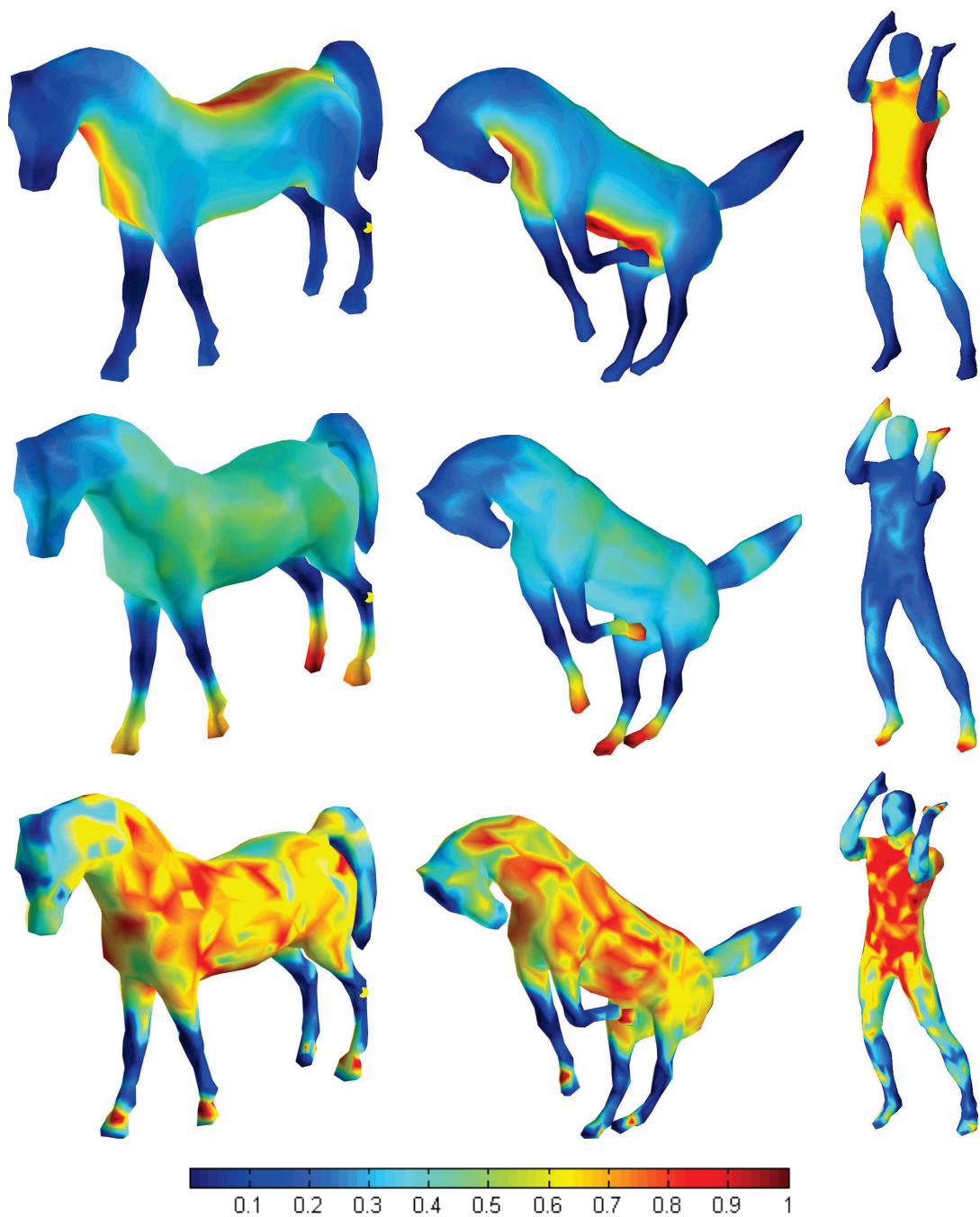
FIGURE 3.4: Normalized \chi^2 -distance between a reference point (yellow colored on the horse's back left leg) and other surface points using different signatures. Top row: heat kernel. Middle row: wave kernel. Bottom row: cubic spline wavelet kernel with R = 2 .
