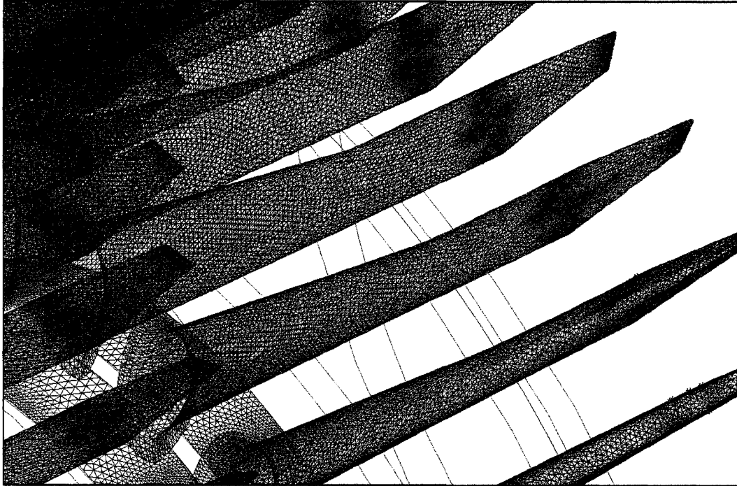
Fig 4.3.3: Detail of mesh on the secondary premix fuel arms.
