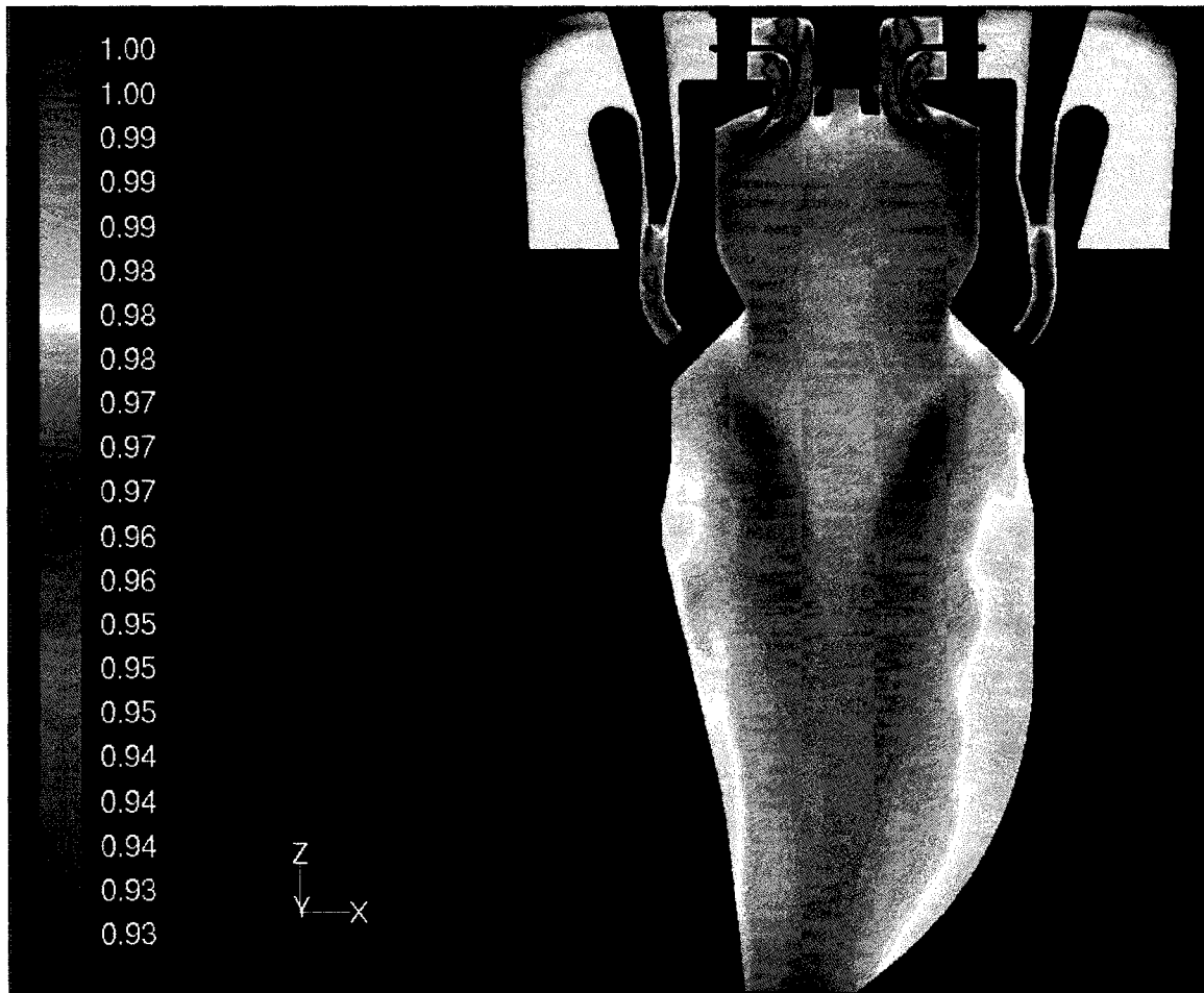
Fig 5.3.1: LES averaged temperature contours (cold fuel hot air).
