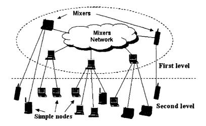
Figure 4.5. Two-level overlay network for mixing
