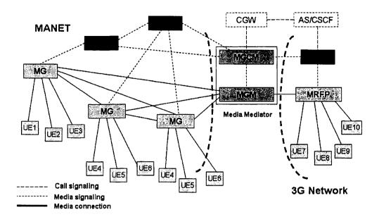
Figure 7.2. Media Handling Architecture for MCNs
