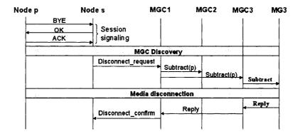
Figure 5.3. Disconnecting a simple node
