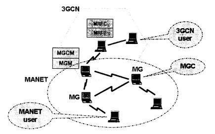
Figure 8.18. MCN test bed architecture
