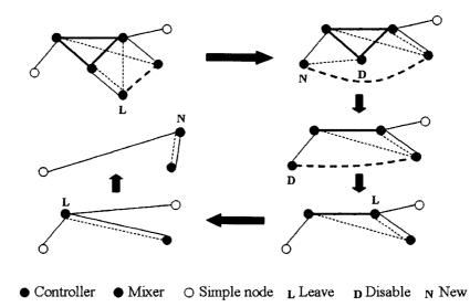
Figure 6.5. Network shrinkage
