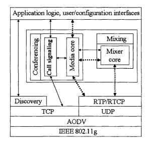
Figure 8.1. DMA prototype architecture
