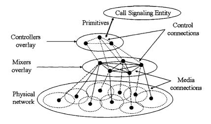
Figure 4.1. Two-overlay architecture
