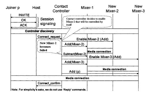
Figure 6.4. Enabling an alternate new mixer when a newly enabled mixer suddenly fails
