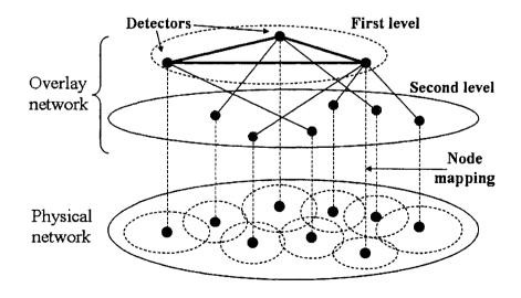
Figure 6.7. Overlay-based failure detection architecture
