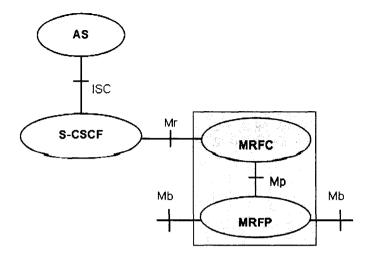
Figure 3.6. Architecture of the MRF
