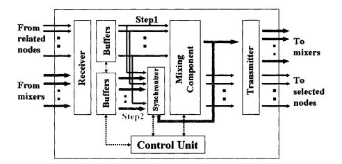
Figure 4.8. Mixer core functional architecture
