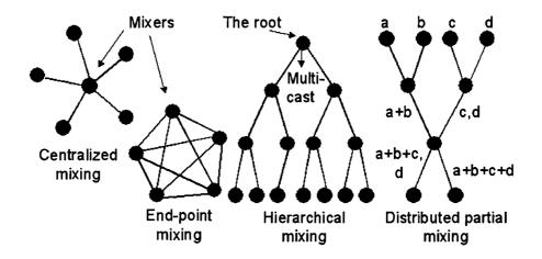
Figure 3.1. Existing mixing architectures
