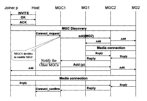
Figure 5.6. Enabling a new MG
