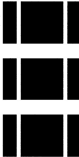
Figure 4.18 – The light field masks which is used for patterning the PVDF sample
