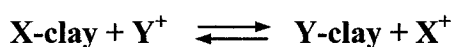
Figure 2.3. Exchange occurs between the ions of the clay ( \text{X}^+ ) and those of the electrolyte ( \text{Y}^+ ) [39]
