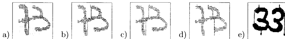
Figure 11: Drop fall algorithms: (a) Top left, (b) Bottom left, (c) Top right, (d) Bottom right, (e) Some examples of errors produced by a wrong starting point selected by the drop fall algorithm.
