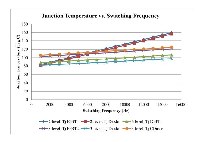
Figure 3.20: Junction Temperature for all the Devices in Two- and Three-level Inverters for a Torque of 180 Nm and a Speed of 3500 RPM
