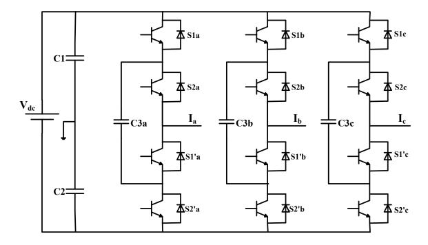
Figure 1.5: Three-phase Capacitor-Clamped Multilevel Inverter
