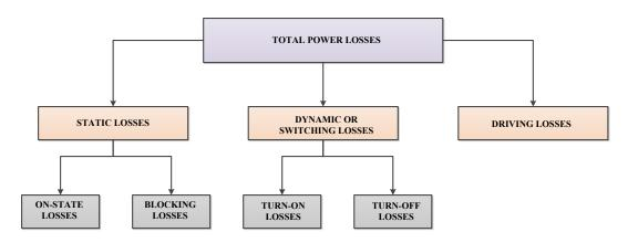
Figure 3.7: Losses Associated with a Power Electronic Switch
