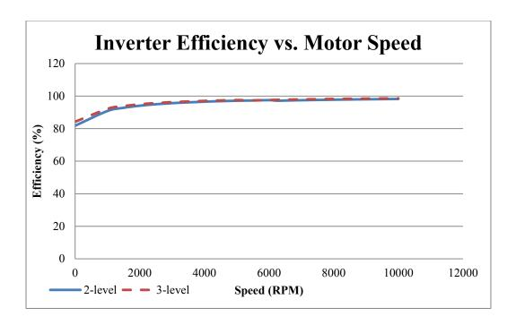
Figure 3.22: Efficiencies of Two and Three-level Inverters for Transient Region of Operation of the Motor
