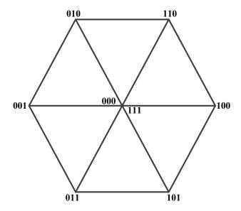
Figure 5.2: Output Voltage Space Vectors of a Three-Phase Two-level Inverter
