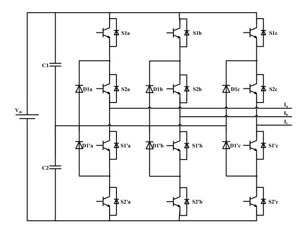
Figure 1.4: Three-phase, Three-level Neutral Point-Clamped Inverter
