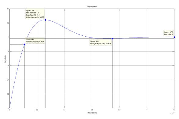
Figure 4.8: Step Response of the Closed Loop Transfer Function for Neutral-Point
