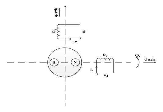
Figure 2.1: Model of PMSM in 'dq' or Rotor Reference Frame
