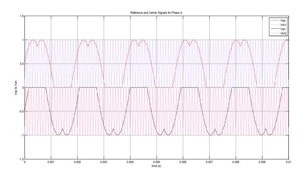
Figure 4.5: Positive and Negative Reference Signal for Phase 'A' of Three-level Inverter
