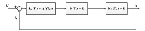
Figure 2.10: Closed-loop for Current Control
