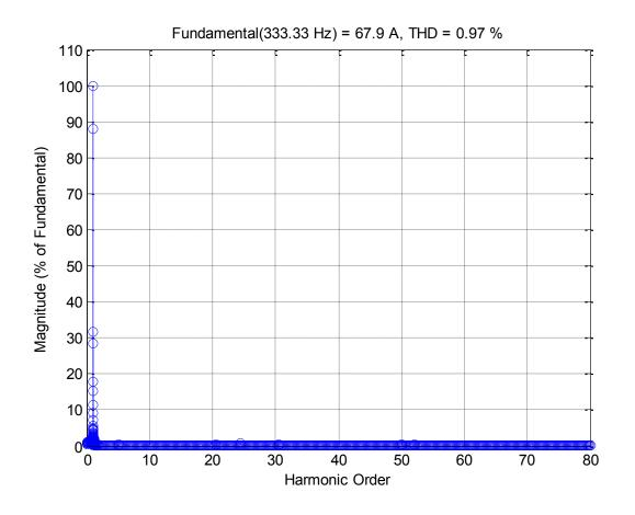
Figure 5.11: Output Current THD for Three-level Inverter at the Switching Frequency of 8.5 kHz using SVM
