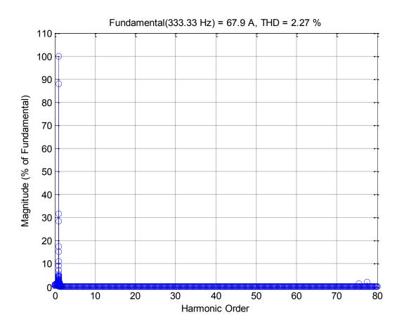
Figure 4.16: Output Current THD for Two-level Inverter at Switching Frequency of 26.5 kHz
