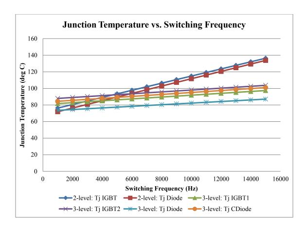
Figure 3.21: Junction Temperature for all the Devices in Two- and Three-level Inverters for a Torque of 127 Nm and a Speed of 7500 RPM
