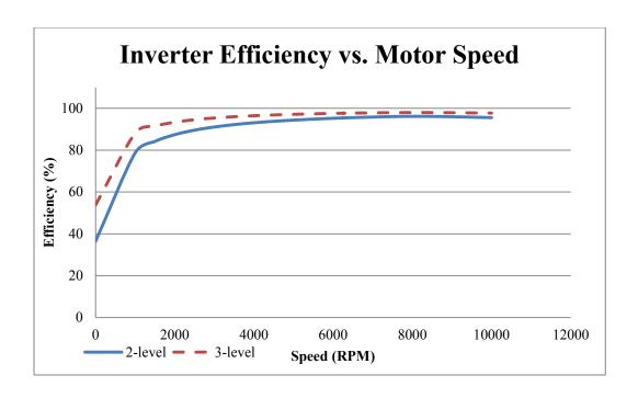
Figure 3.23: Efficiencies of Two and Three-level Inverters for Continuous Region of Operation of the Motor at 20 kHz Switching Frequency
