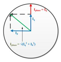
Figure 2.5: Torque and Flux-Producing Components of the Stator Phase Current
