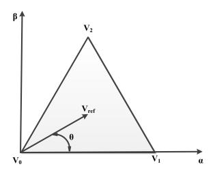
Figure 5.3: Sector 1 of a Two-Level Inverter
