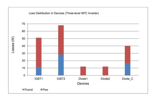
Figure 4.19: Loss Distribution in Three-level Inverter
