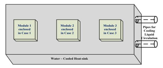
Figure 3.3: Multiple Layer Structure for a Liquid-Cooled Power Electronic Converter
