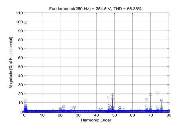
Figure 4.15: Line Voltage THD for Three-level Inverter with CB-SVM
