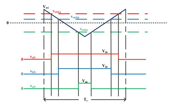
Figure 4.2: Gating Signal Generation in a Switching Period for One Leg of a Two-level
