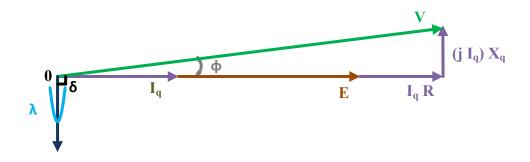
Figure 2.3: Phasor Diagram of Single-Phase of PMSM before Introducing Field-Weakening
