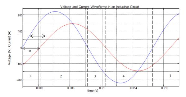
Figure 3.9: Steady-State, Load Voltage and Load Current Waveforms for an Arbitrary RL-load
