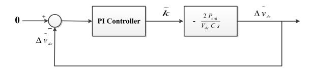
Figure 4.6: Closed-loop for the Neutral-Point Voltage Control
