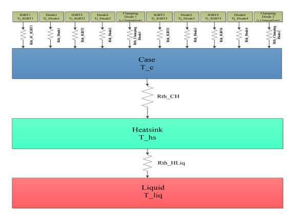
Figure 3.6: Thermal Equivalent Circuit for One Module of Three-level NPC Inverter
