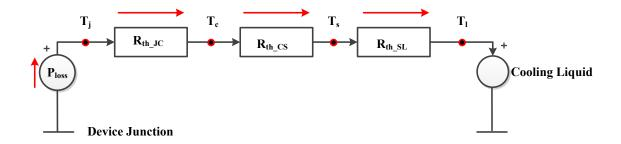
Figure 3.4: Electrical Equivalent of the Thermal Circuit of a Liquid-Cooled
