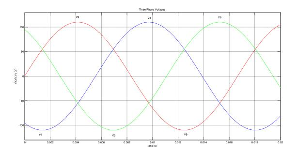
Figure 5.1: Three-Phase Balanced Voltage Supply
