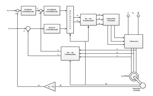
Figure 2.8: Field-Oriented Control of PMSM
