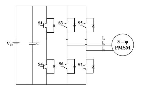
Figure 3.1: Conventional, Two-level Inverter
