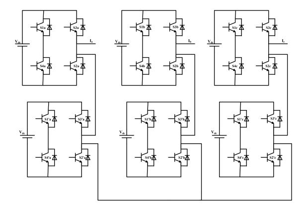
Figure 1.3: Three-phase Cascaded H-Bridge Multilevel Inverter
