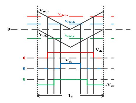
Figure 4.3: Gating Signal Generation in a Switching Period for One-leg of a Three-level
