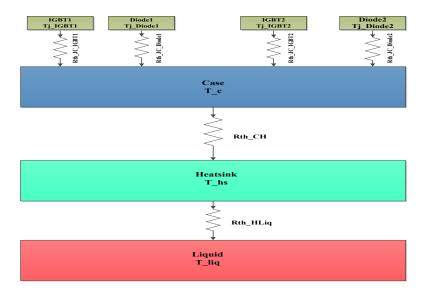
Figure 3.5: Thermal Equivalent Circuit for One Module of Two-Level Inverter
