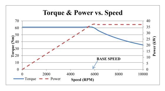
Figure 2.7: Torque & Power as a Function of Speed in the Continuous Region of Operation
