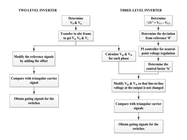
Figure 4.13: Flow Chart for CB-SVM of Two and Three-level Inverters
