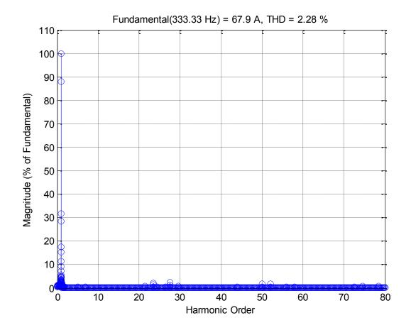
Figure 4.17: Output Current THD for Three-level NPC Inverter at the Switching Frequency of 8.5 kHz using CB-SVM
