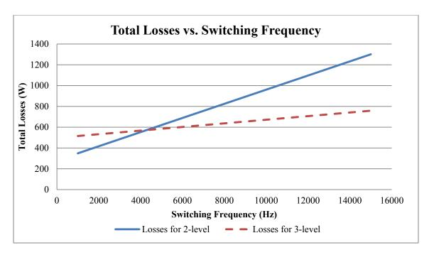
Figure 3.18: Total Losses as a Function of Switching Frequency for Two- and Three-level Inverters for a Torque of 180 Nm and a Speed of 3500 RPM
