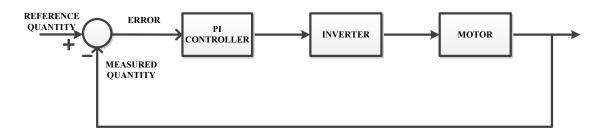
Figure 2.9: Simplified, Closed-loop Block Diagram of the System
