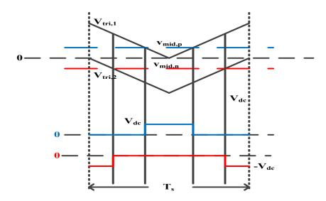
Figure 4.4: Decomposition of a Reference Signal in a Switching Period
