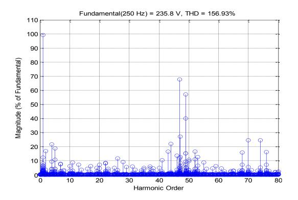
Figure 5.9: Line Voltage THD for Two-level Inverter with SVM
