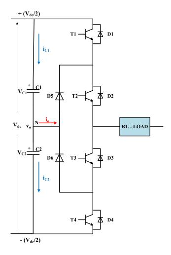
Figure 3.26: Three-level Neutral-Point Clamped Inverter with the DC-link Capacitors
