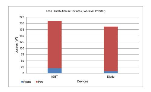
Figure 4.18: Loss Distribution in Two-level Inverter
