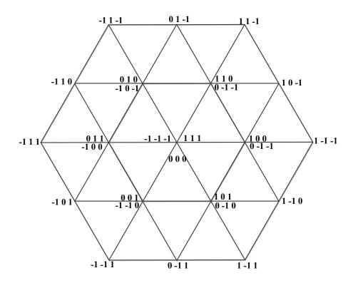
The zero vectors (magnitude '0') are present at the center of the hexagon while the small vectors (magnitude ' $\frac{1}{3}$ ') are the ones that are present in pairs at the vertices of the inner hexagon. The medium vectors (magnitude ' $\frac{1}{\sqrt{3}}$ ') are the ones that lie in between the mid-points of the two consecutive vertices of the outer hexagon and the large vectors (magnitude ' $\frac{2}{3}$ ') are those that are present at the vertices of the outer hexagon. All the
