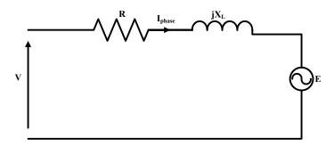
Figure 2.2: Per-phase Equivalent Circuit of a Permanent Magnet Synchronous Machine
