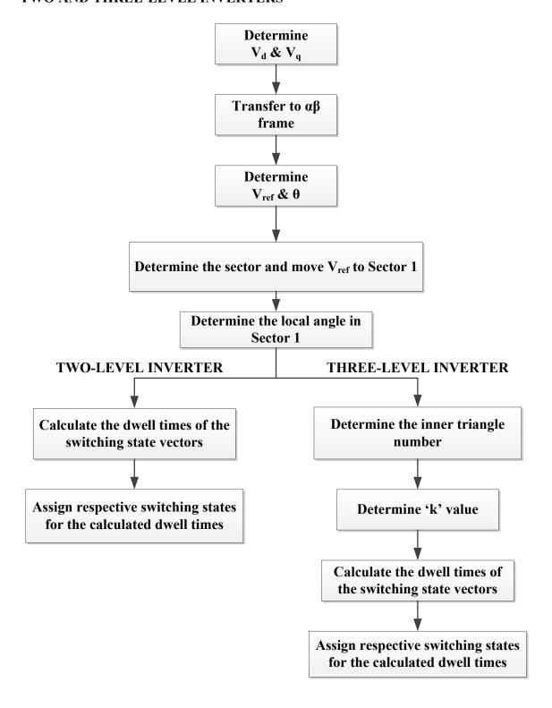
Figure 5.8: Flow Chart for SVPWM of Two and Three-level Inverters
