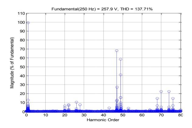
Figure 4.14: Line Voltage THD for Two-level Inverter with CB-SVM
