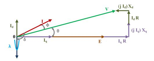
Figure 2.4: Phasor Diagram of Single-Phase of PMSM after Introducing Field-Weakening
