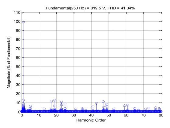
Figure 5.10: Line Voltage THD for Three-level Inverter with SVM
