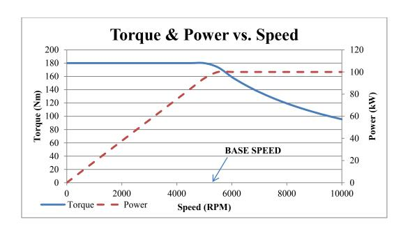
Figure 2.6: Torque & Power as a Function of Speed in the Transient Region of Operation
