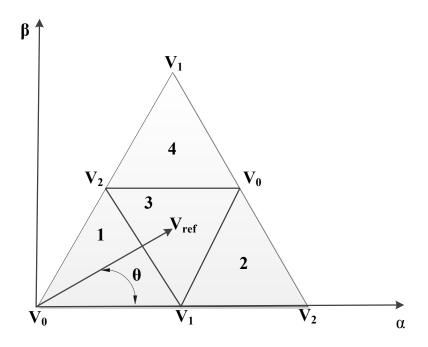
Figure 5.5: Sector 1 of a Three-Level Inverter
