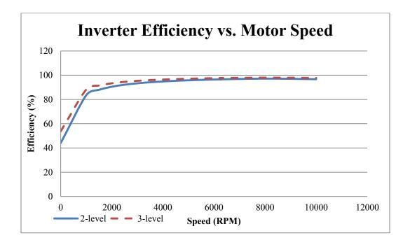
Figure 3.24: Efficiencies of Two and Three-level Inverters for Continuous Region of Operation of the Motor
