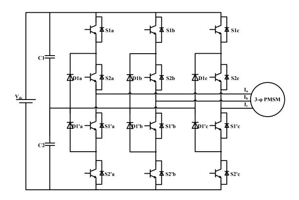
Figure 3.2: Three-level Neutral Point-Clamped Inverter
