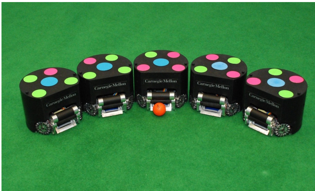
Figure 2.4 Robot soccer players distinguished by different color signs (image from Carnegie Mellon University robot soccer team)
