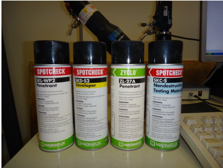
Figure 3.2 FPI chemicals: Water Washable Penetrant, Developer, Solvent Removable Penetrant and Solvent Cleaner (From left to right)
