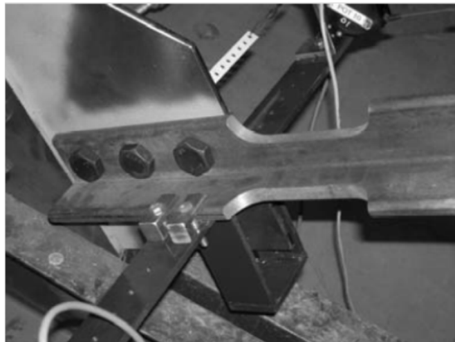
Figure 2.3: Configuration of a cut-out ductile fuse (Desjardins and Légeron, 2010)
