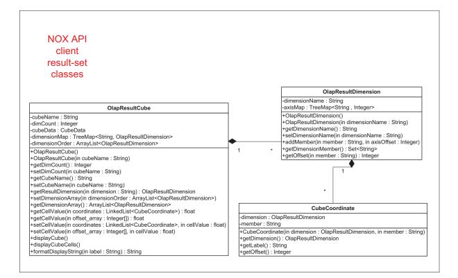
Figure 35: UML class diagram for the NOX API Result Set classes
