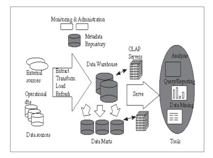
Figure 2: Typical data warehouse architecture
