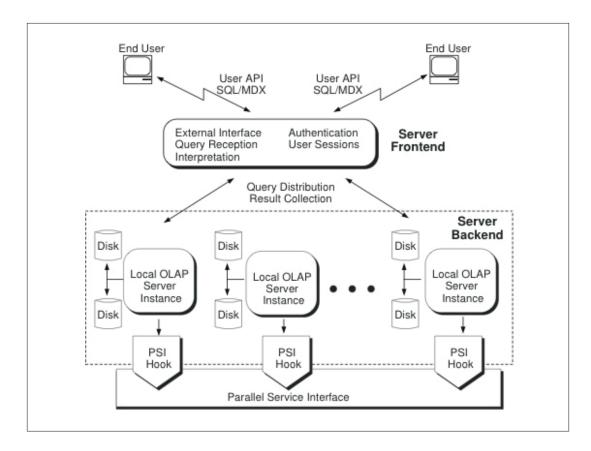
Figure 13: The core architecture of the parallel Sidera OLAP server [EDD<sup>+</sup>07]
