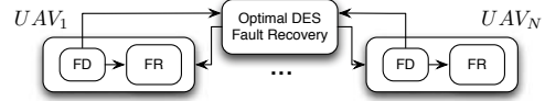
Fig. 1. Our proposed hybrid framework for a team of N UAVs (Legend: FD = fault diagnosis and FR = fault recovery).
