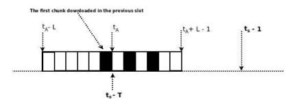
Figure 5.2: The buffer when  $t_A = t_s - T$ , after downloading the first chunk
