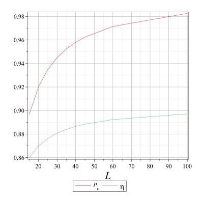
Figure 3.14: L The Effect of Buffer length on  $Pc, \eta$
