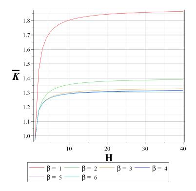
Figure 3.19:  $\bar{K}$  as a function of upload bandwidth  $\beta$
