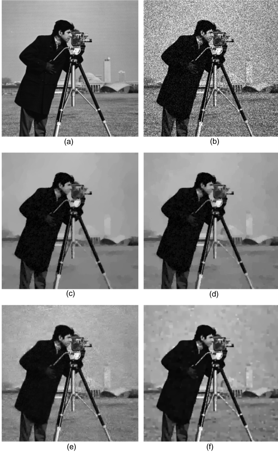
Figure 4.6: The perceptual quality of the processed image Cameraman : (a) Noiseless image. (b) Noisy image when f_M^* = 30 . (c) Image denoised using TV-KL with \alpha = 2.80 . (d) Image denoised using SPIRAL-TV with \tau = 0.30 . (e) Image denoised using PURE-LET. (f) Image denoised using proposed method with \chi_0 = 1.02 .
