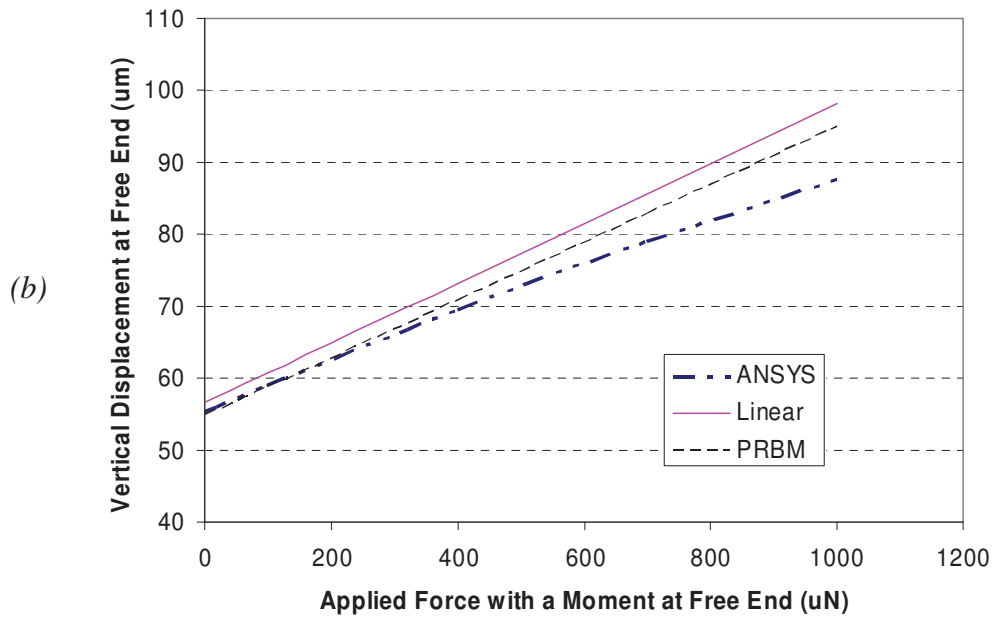
Figure 2.13 Different load-deflection curves of a cantilever at free end are simulated using linear beam theory, PRBM and FEM software: the curves in (a) are resulted from a range of moment with a fixed force; and the curves in (b) are resulted from a range of force with a fixed moment.
