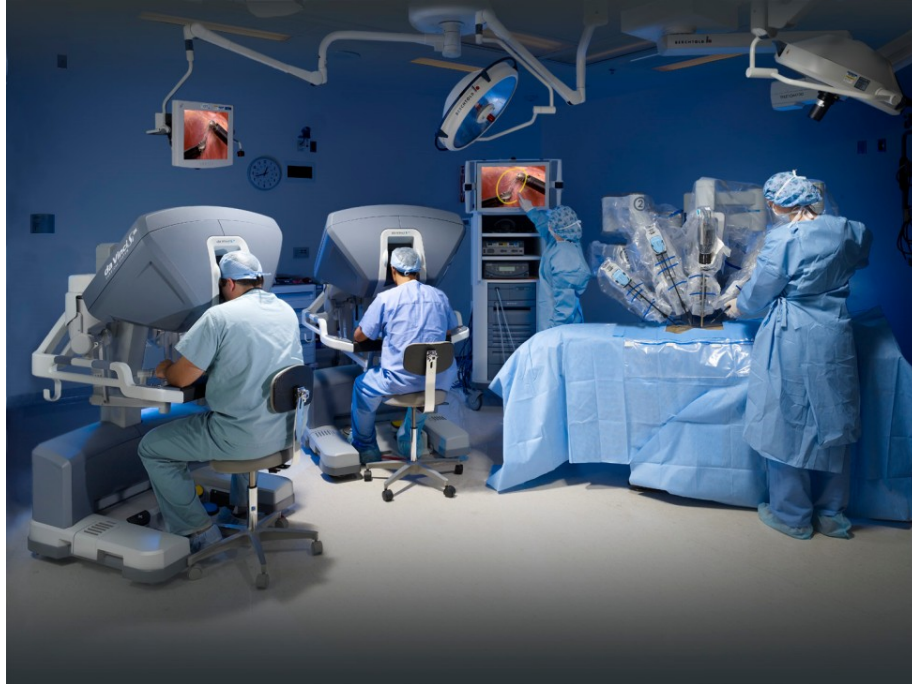
Figure 1-2: Photograph of a surgical operating room featuring the da Vinci Surgical System. This photograph is the courtesy of Intuitive Surgical Inc. ( http://www.intuitivesurgical.com ), ©[2011] Intuitive Surgical, Inc. [5]. The system comprises one surgical robot, two surgeon consoles, one patient cart, and one vision cart.
