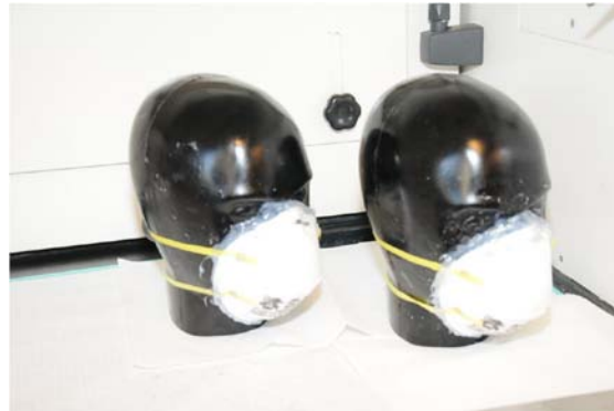
Figure 1. Sealed N95 FFR on the manikin head.
