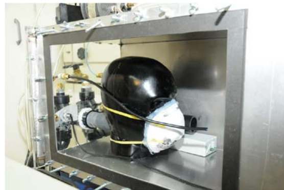
Figure 2. Manikin head with the sealed N95 FFR in the challenge chamber.
