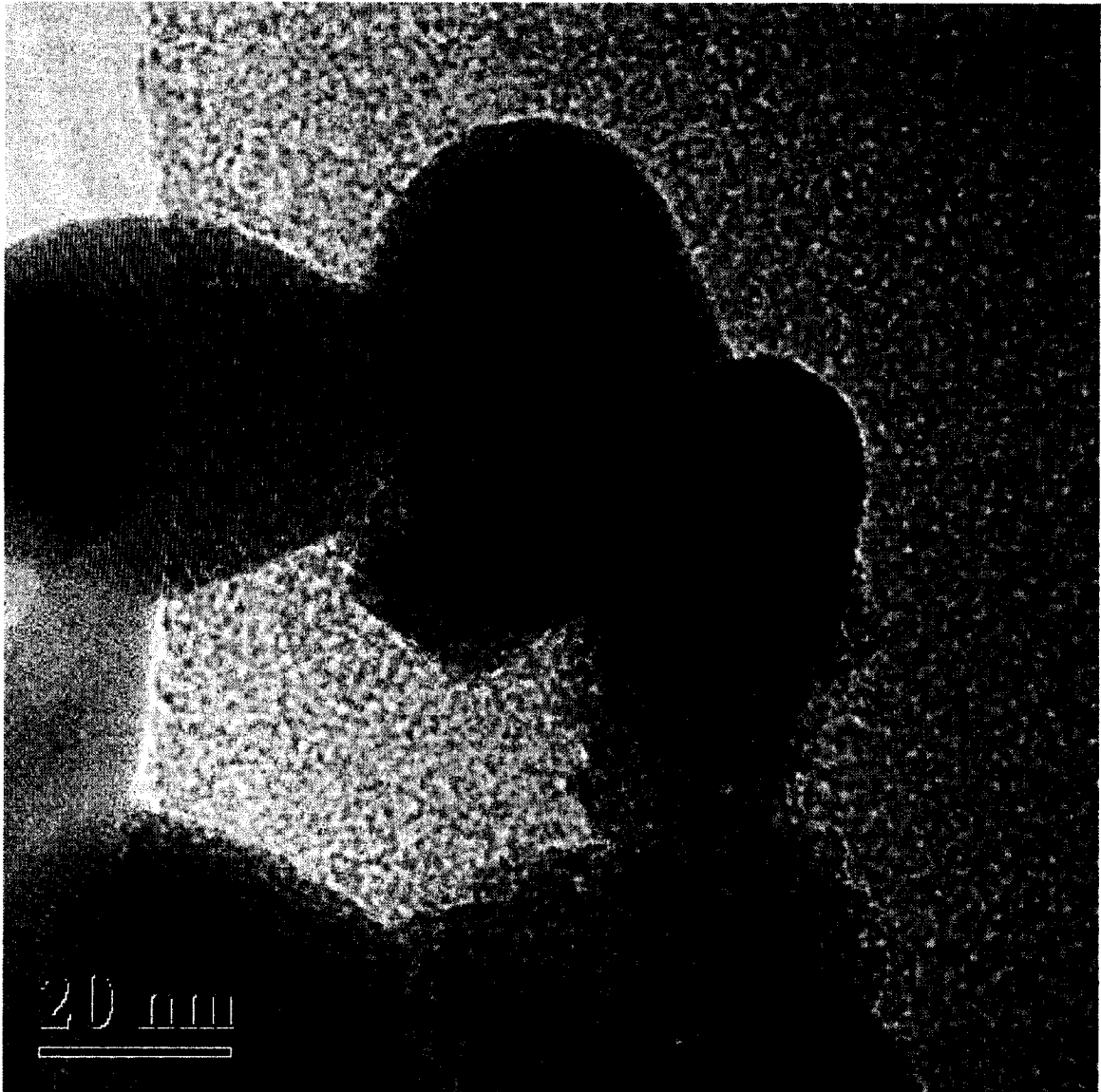
Figure 3. 1. TEM Micrograph of gadolinium gallium garnet nanocrystals
