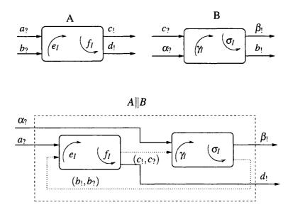
Figure 2.6: Composition of compatible I/O automata.
