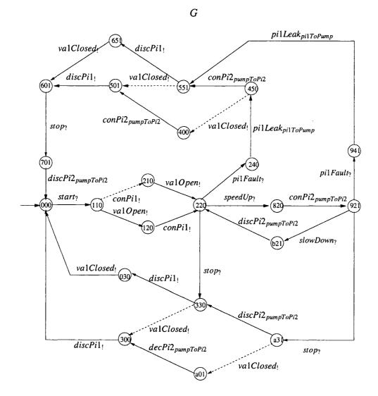
Figure 5.5: Pump system: the entire plant behavior. Illegal events are shown by dashed lines.
