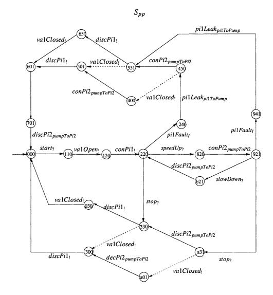
Figure 5.8: Pump system: the plant under the supervision of  $S_{pp}$ . Events that are illegal but uncontrollable to  $S_{pp}$  (i.e., should be disabled by  $S_{pi1}$ ) are shown by dashed lines.
