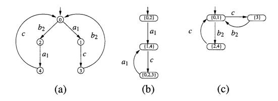
Figure 2.3: The observer automata of a DES: (a) the plant G; (b)  $Obs_1(G)$ ; (c)  $Obs_2(G)$  (adopted from [1]).
