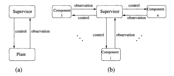
Figure 2.1: Architecture of centralized supervisory control.
