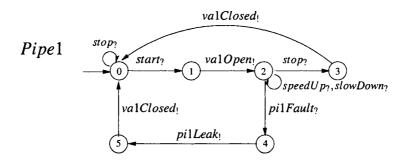
Figure 5.2: Pump system: pipe 1.
