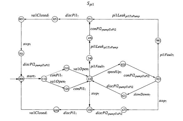
Figure 5.9: Pump system: the plant under the supervision of  $S_{pi1}$ . Events that are illegal but uncontrollable to  $S_{pi1}$  (i.e., should be disabled by  $S_{pp}$ ) are shown by dashed lines.
