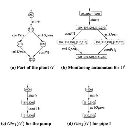
Figure 5.10: Observer and monitoring automata for a selected part of the plant.
