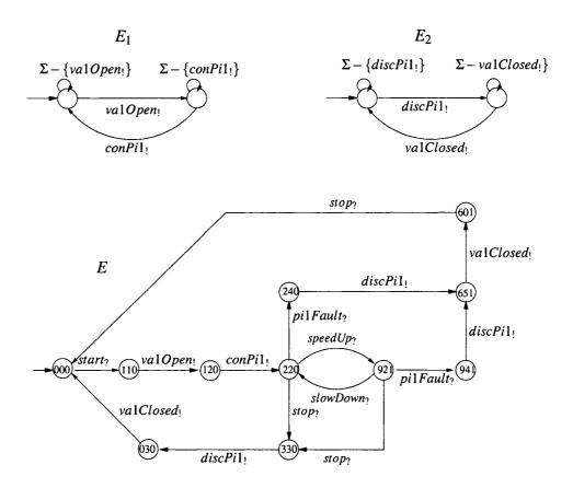
Figure 5.6: Pump system: the service specification.
