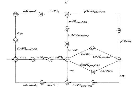
Figure 5.7: Pump system:  $E' = \sup \mathscr{C}(P_{ex}^{-1}(E) \cap L(G)).$
