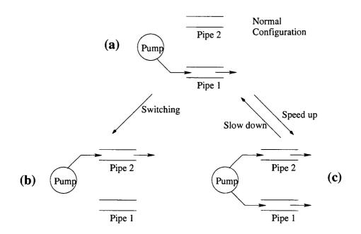
Figure 5.1: Pump system: the system architecture.
