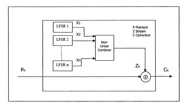
Figure 1.4: LFSR-based stream cipher
