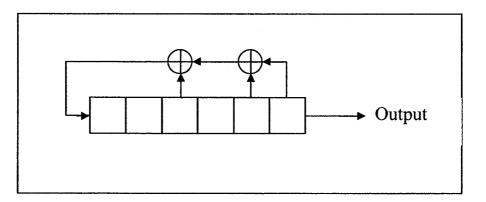
Figure 1.3: An example for a 6-bit linear feedback shift register
