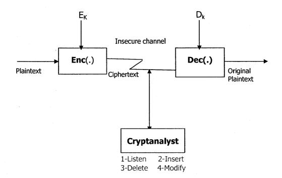
Figure 1.1: A typical secure communications system
