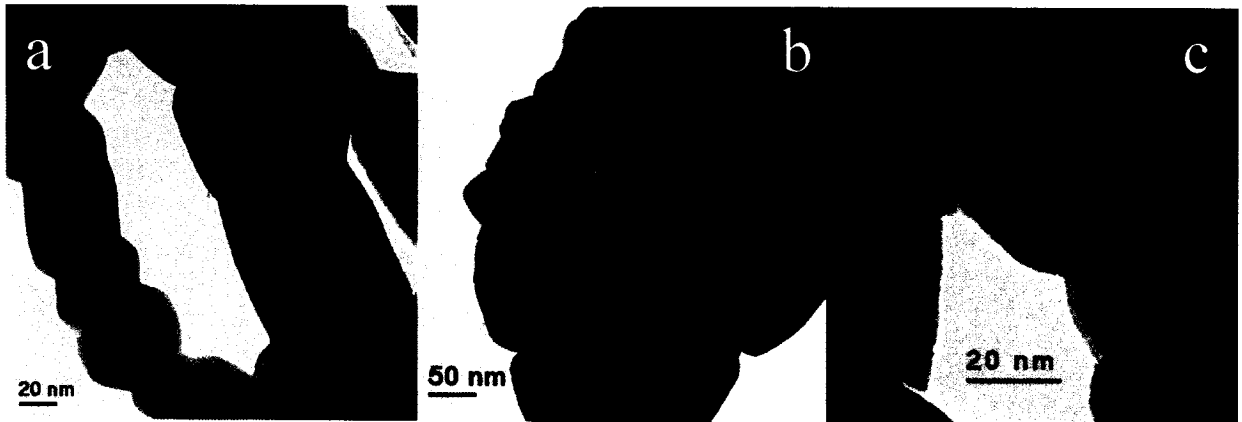
Figure 5.7: TEM micrographs of \text{Lu}_2\text{O}_3 nanocrystals prepared via propellant synthesis.
