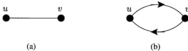
Figure 2: An edge (u, v) in an undirected graph (a) becomes two edges (u, v) and (v, u) in a symmetric digraph (b).
