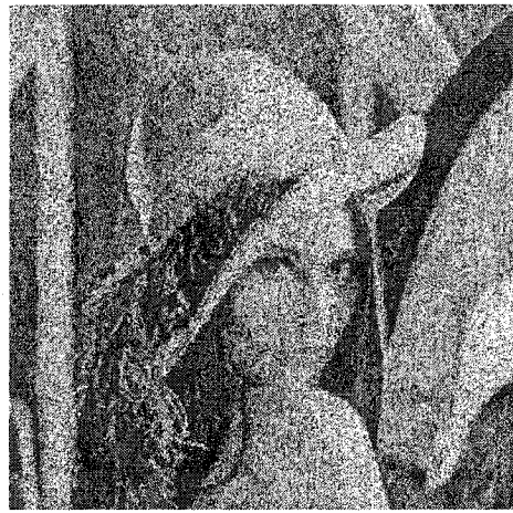
(c) JPEG compression, PSNR = 19.79 dB, bpp = 0.37
