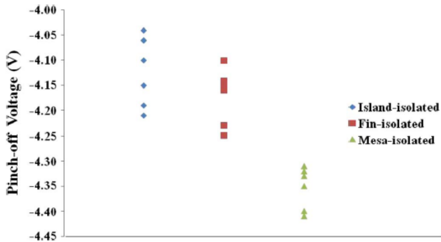
Figure 2.7: Scatter plot of the variation of the pinch-off voltage among the three categories of devices.
