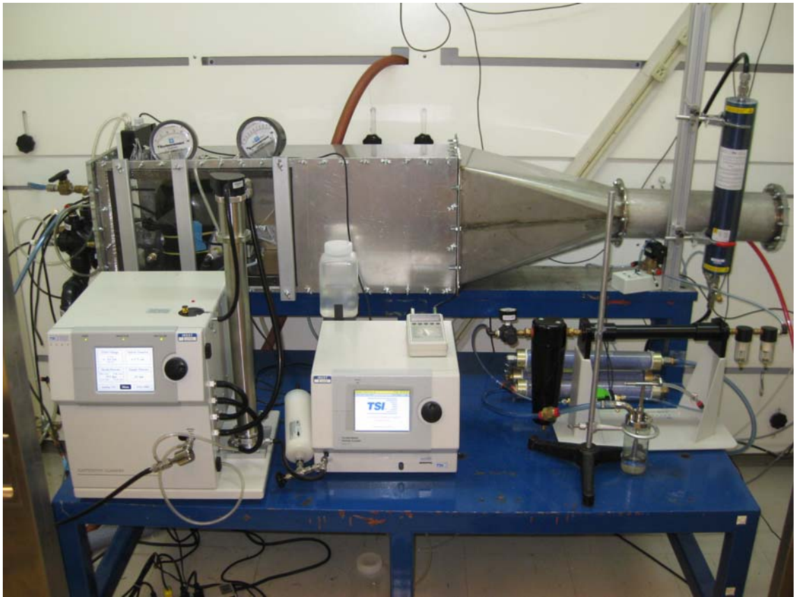
Figure 3-3: Schematic of the test system used to challenge N95 respirators against poly-disperse aerosols.
