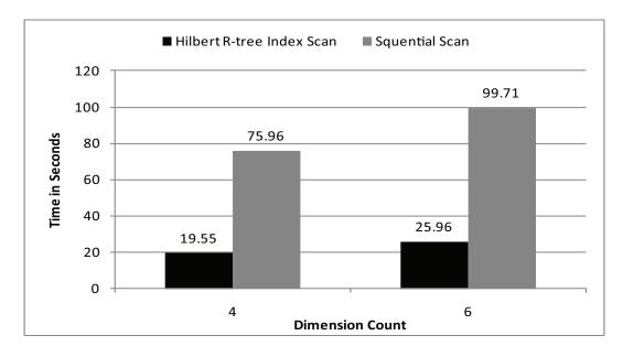
Figure 6.6: Sequential Scan versus Hilbert R-Tree index Scan.
