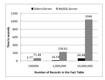
Figure 6.13: Sidera Query Engine against MySQL Engine as the number of records increases.
