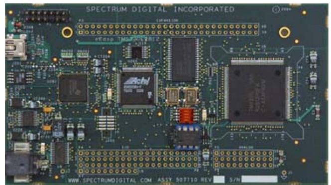
Fig. 9. PCB of the eZdsp R2812 DSP controller.
