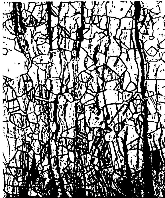
Fig. 48. An optical micrograph of a tangential section of a 301W specimen deformed at 1100^{\circ}\text{C} , 5 \text{ s}^{-1} shows broad surface cracks which are most marked at opposite edges where the section is closest to the surface and almost disappear in the middle except for their deepest tips. X 150.
