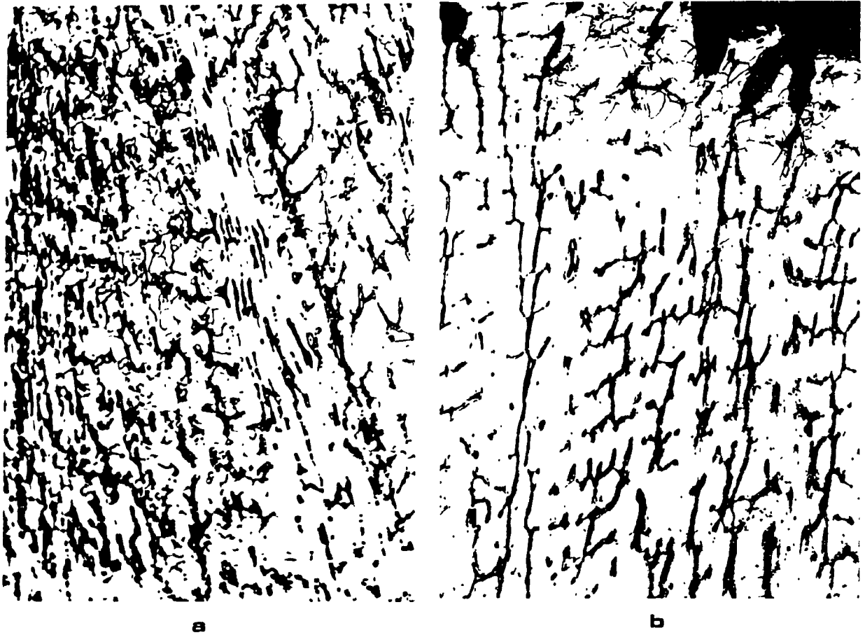
Fig. 53. Optical micrograph of a) a longitudinal section of 317C deformed at 1000^{\circ}\text{C} , 0.1 \text{ s}^{-1} showing cracks parallel to the stringers of \delta phase. X 200, and b) a tangential section of 316C specimen deformed at 1000^{\circ}\text{C} , 5 \text{ s}^{-1} showing \delta stringers in elongated form connected by pores and leading to surface grooves. X 200.
