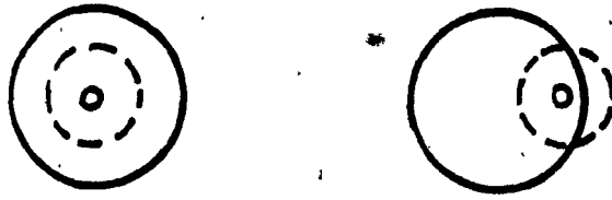
Figure 21. A representation of how the spatial energy is changed as the test flash is moved from the center to the edge of the background.
