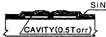
Figure 1.26 A diaphragm with a point support at the center [adopted from Sugiyama et al [171]]
