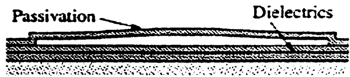
b) clamped-clamped beam of a 2 \mu m CMOS process [Adopted from Paul [135]]
