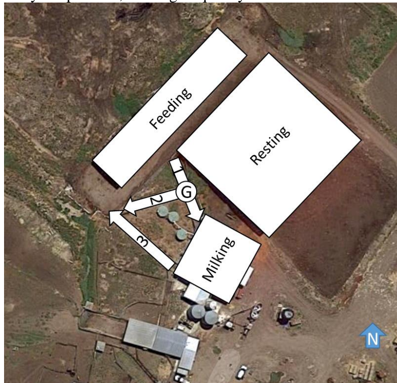
Figure 5-2 Layout of farm traffic. The letter “1” indicates the passageway toward milking station; the letter “G” indicates the drafting gate to control animal access to milking station; the letter “2” indicates the passageway of rejected cows, and the letter “3” indicates the general passageway of existing milking station. No limitation of access or forced movement between feeding and resting area. Adapted from google map
