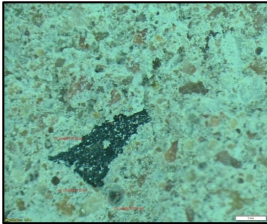
(a) 0% (average pore diameter: 454 \mu m)
