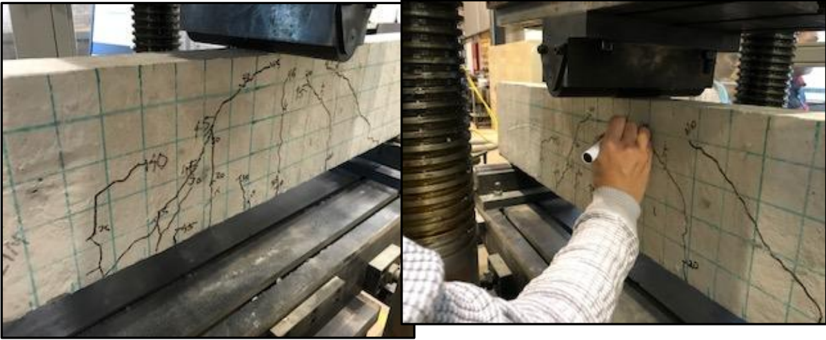
Figure19: Load-Displacement behaviour and failure behaviour of beam 1 without oil and beam 2 with oil contamination
