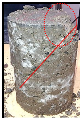
(Shear failure) with fracture conically 10%
