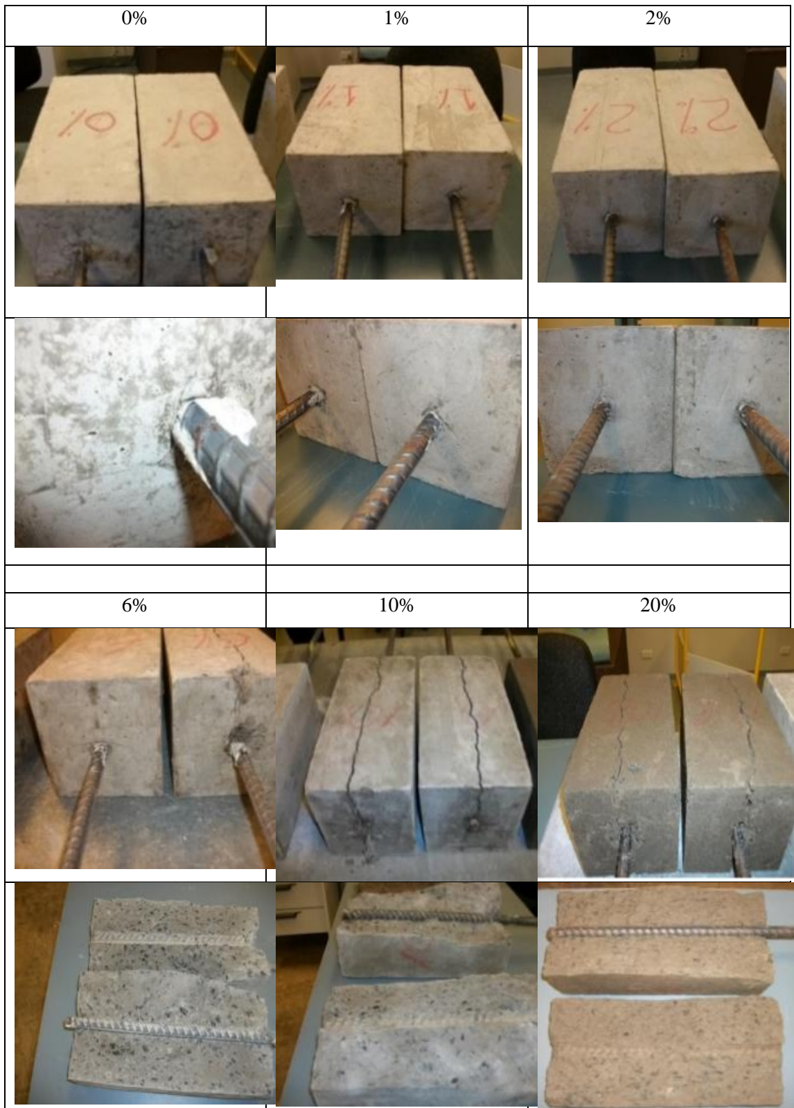
Figure 17: Failure modes of different samples due to pull out test
