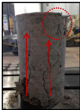
Splitting with fracture conically 0%
