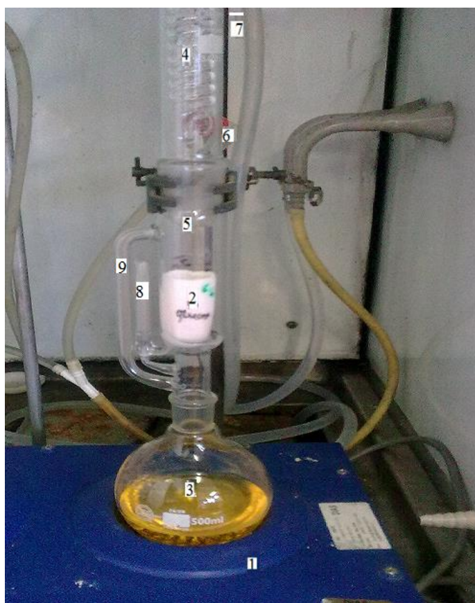
Figure 4.4 Soxhlet extractor using hexane as solvent
