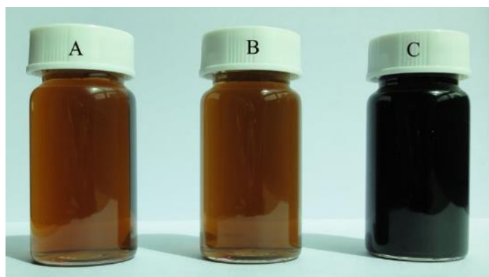
Figure 3 - 5 The color change of exfoliated GO suspension in a different procedure. (A) is GO; (B) is GO heated at 90 °C for 2 h; (C) is GO mixed with the K 2 CO 3 solution and heated at 90 °C for 2 h.
