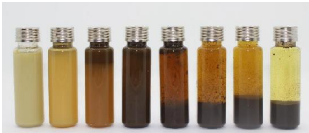
Figure 5 - 23 The different amount of PDDA/AgNPs/RGO added into NR latex. From left to right the content of AgNPs/RGO was added 0.1 vol.%, 0.29 vol.%, 0.52 vol.%, 1.01 vol.%, 1.65 vol.%, 2.06 vol.%, 2.87 vol.%, and 4.03 vol.%, respectively.
