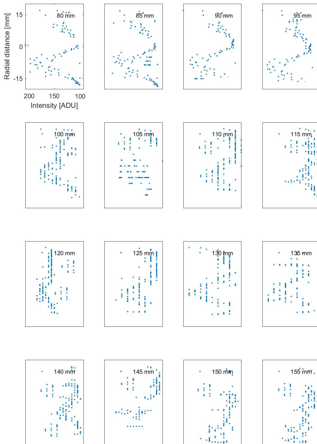
Figure 8.21: Intensity variation within the ejector duct at locations between 80 and 155 mm from the nozzle exit at 220 kPa, 1.6 kPa and 5.7 kPa as a primary pressure, secondary pressure and back pressure respectively.
