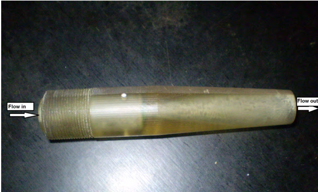
Figure 4.5: Photograph of the primary nozzle produced by the 3D printer.
