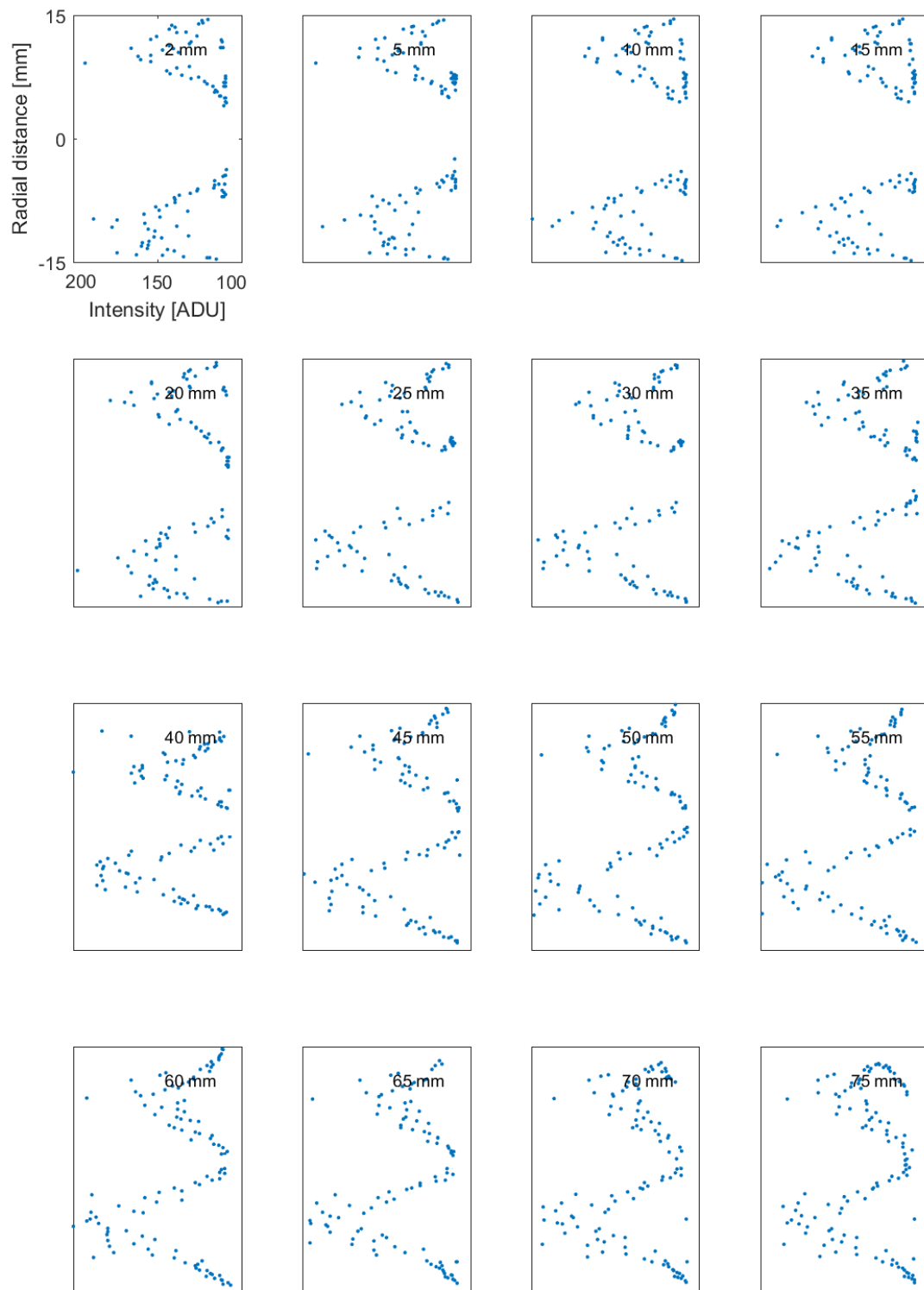
Figure 8.16: Intensity variation within the ejector duct at locations between 2 and 75 mm from the nozzle exit at 200 kPa, 1.6 kPa, 4.8 kPa as a primary, secondary pressure and back pressure respectively.
