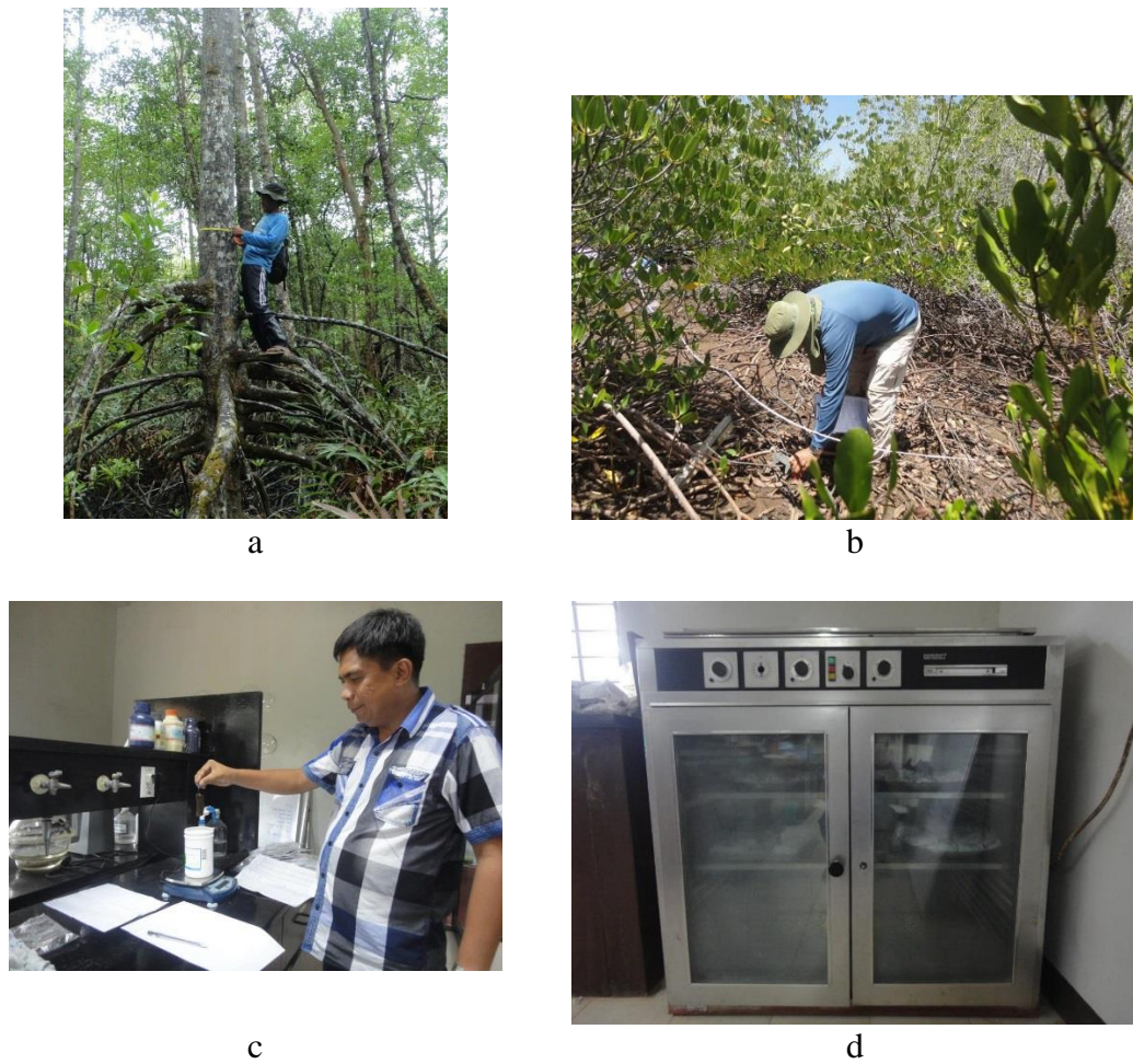
Figure 4.4 Data collection for biomass estimation. a) measuring the tree diameter, b) classifying the diameter of downed woody debris (DWD) using a fuel gauge, c) laboratory works for DWD samples to estimate the volume using water displacement method, and d) oven-drying the DWD samples
