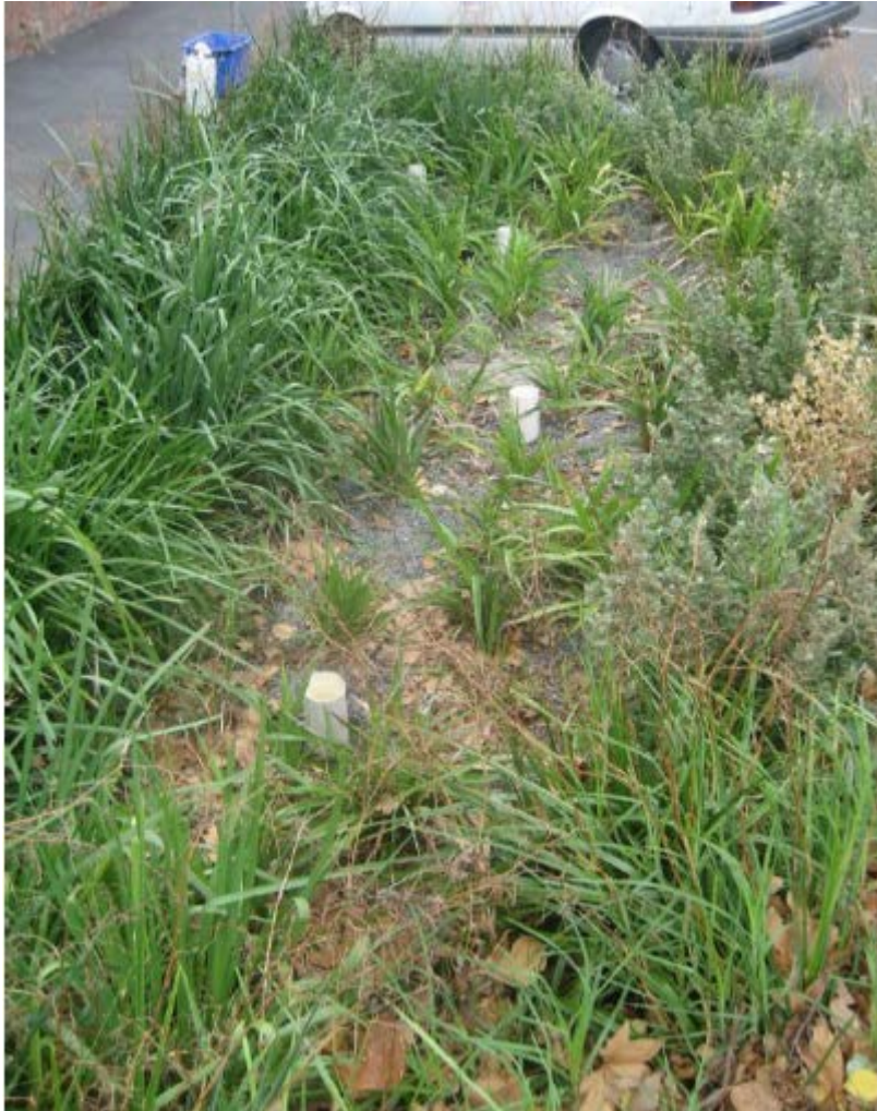
Figure 2.12.3 Single ring test carried out on spatially distributed monitoring points (FAWB 2009a)
