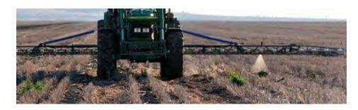
Figure 1.8: Boomspray equipped with Weedseeker technology (reproduced from Cropoptics Australia (2012)).
