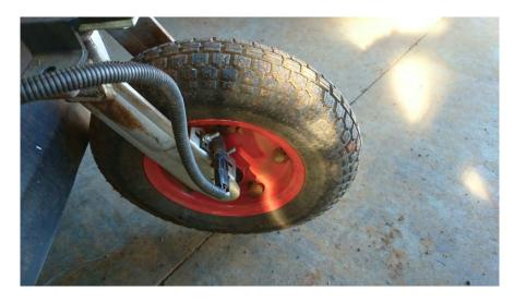
Figure 3.1: The magnetic wheel speed sensor is shown with the sensor and the magnets mounted on the wheel. Each time the magnet passes the sensor, a pulse is created.
