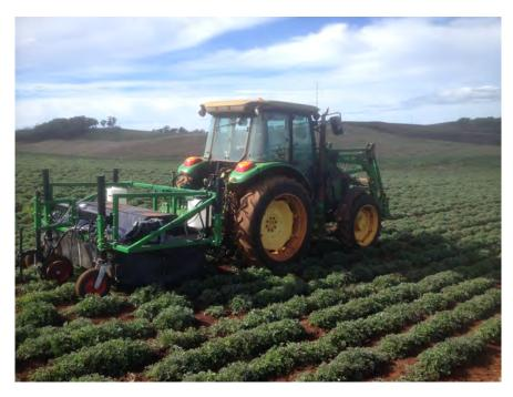
Figure C.2: Tractor and experimental NCEA prototype spot spray system in a crop of first year growing pyrethrum April 2014.
