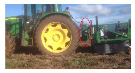
Figure G.1: Image of side shift hitch (in the red ellipse) in position between the tractor at the front and the implement at the rear.
