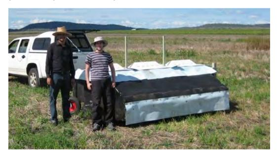
Figure 2.3: Three metre spot sprayer developed for plant identification and spot spraying at the NCEA (McCarthy et al. 2012). Camera and lights are mounted under white plastic covers with a light-restricting cover around the sprayer.
