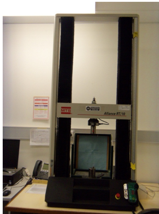
Figure 3.10: 10 KN MTS testing machine.
